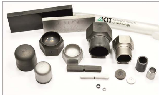
Green parts (dark), finished parts (brighth)
