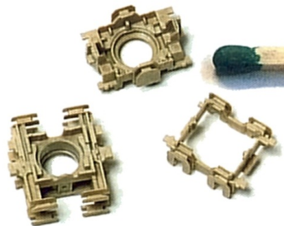
DVD optical pick up system: lens holder
