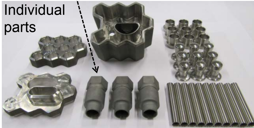
9-finger module (W) for high heat flux (HHF) tests in Efremov
