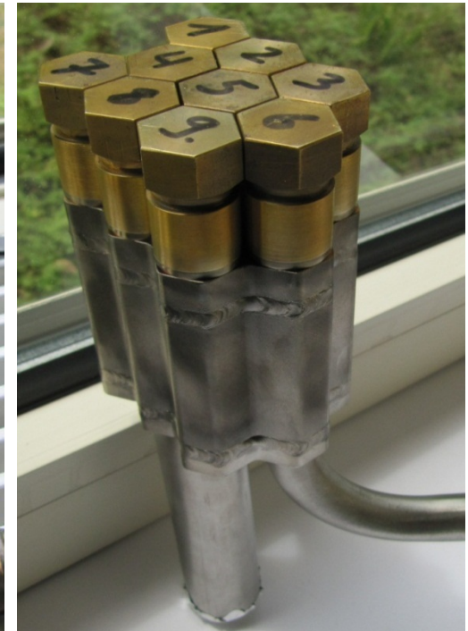
9-finger module (brass) for non-destructive examination (NDE) with SATIR at CEA
