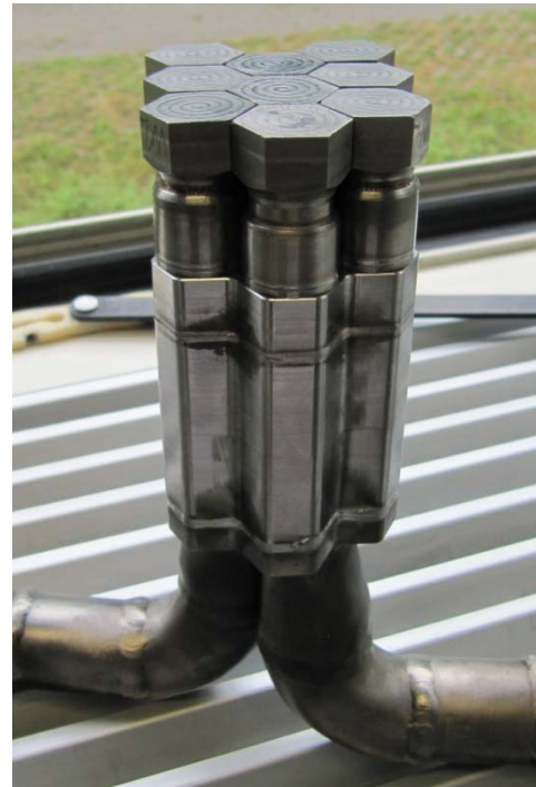
9-finger module (W) for high heat flux (HHF) tests in Efremov
