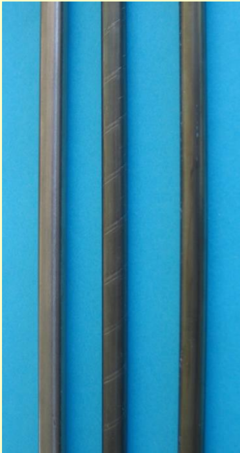
As-received Zry-2 and prototype heater rods
