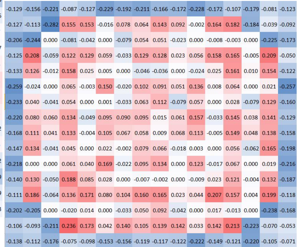
Relative pin power errors DYN3D sp3 (32M) vs. Serpent 2 in per cent
