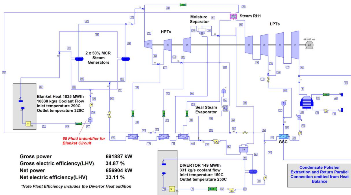
Cycle diagram for Thermoflow model: Rankine cycle of water-cooled reactor (CCFE: <https://user.efda.org/?uid=2MC3W9>)
