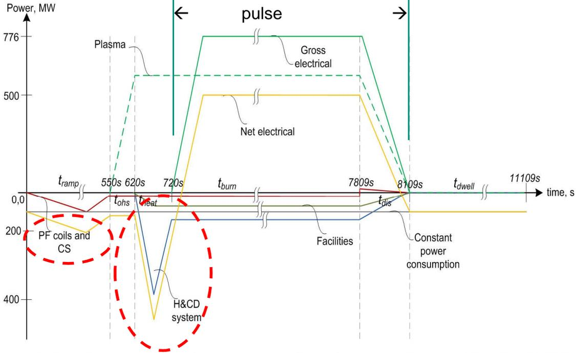
**Figure 3.** Rough estimation of power generation / consumption profiles for DEMO 1 scenario.¶
