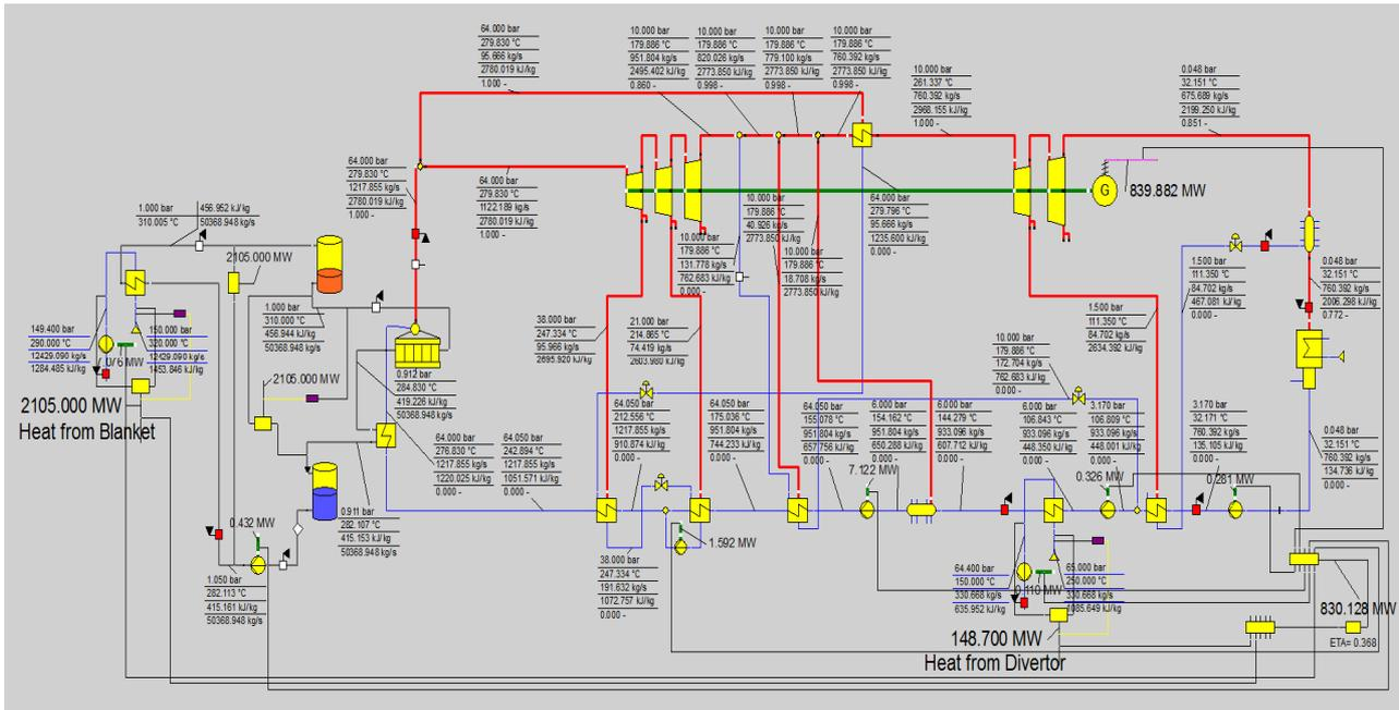
DEMO BoP scheme for water cooled blanket concept with the integrated intermediate heat storage loop as modelled by KIT
