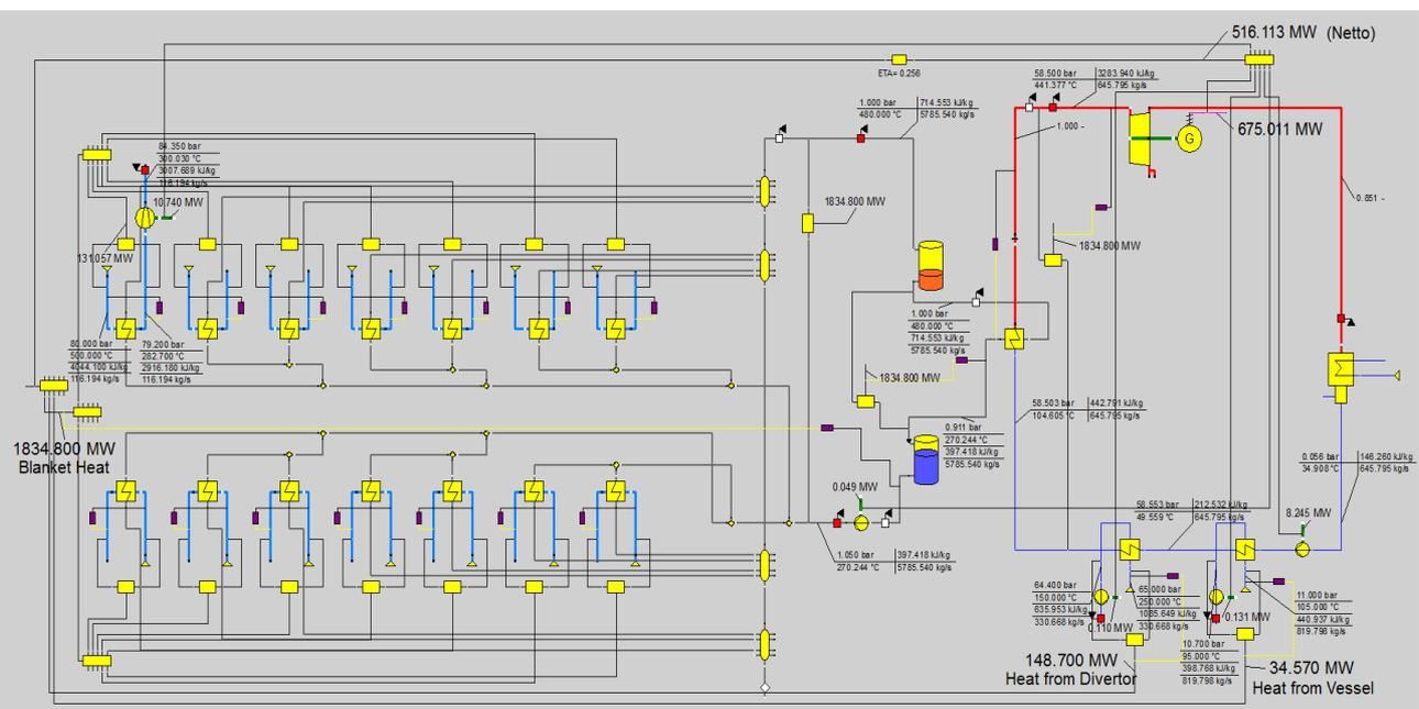
DEMO BoP scheme for helium cooled blanket concept with the integrated intermediate heat storage loop as proposed by KIT
