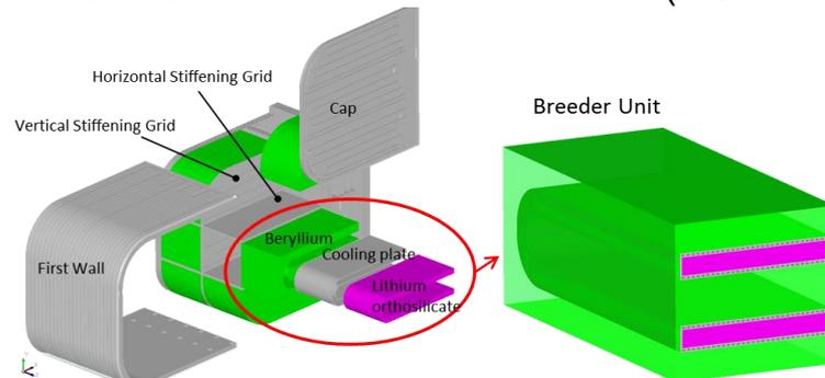
Exploded view of the HCPB TBM test case
