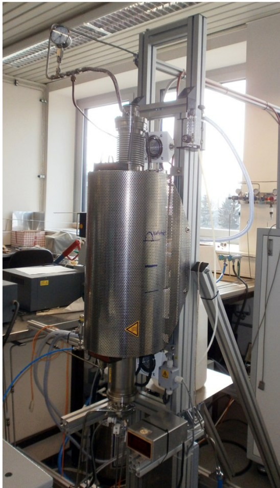
Hydrogenation facility LORA furnace
