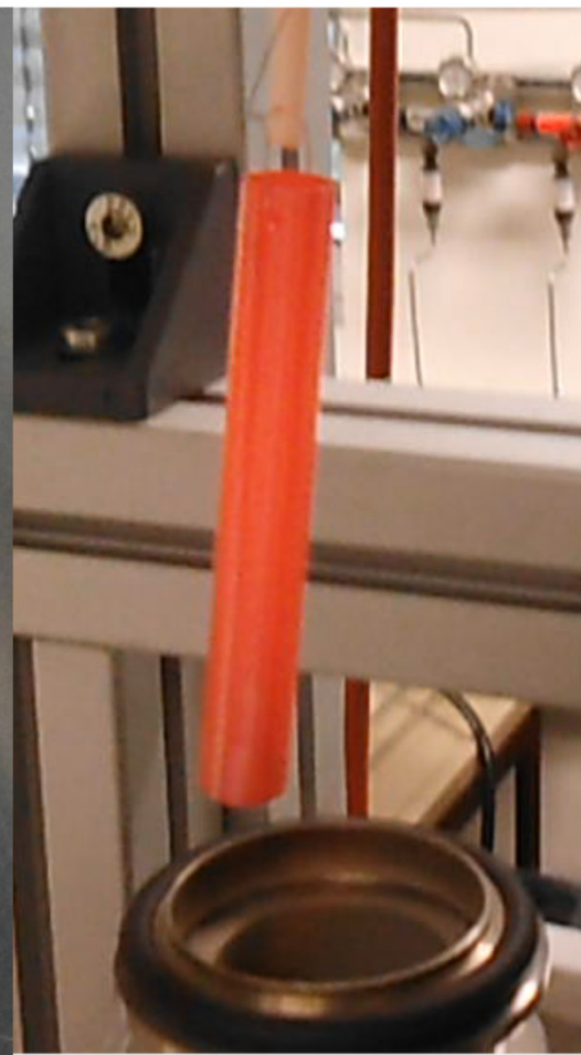
Specimen withdrawal in air after hydrogenation
