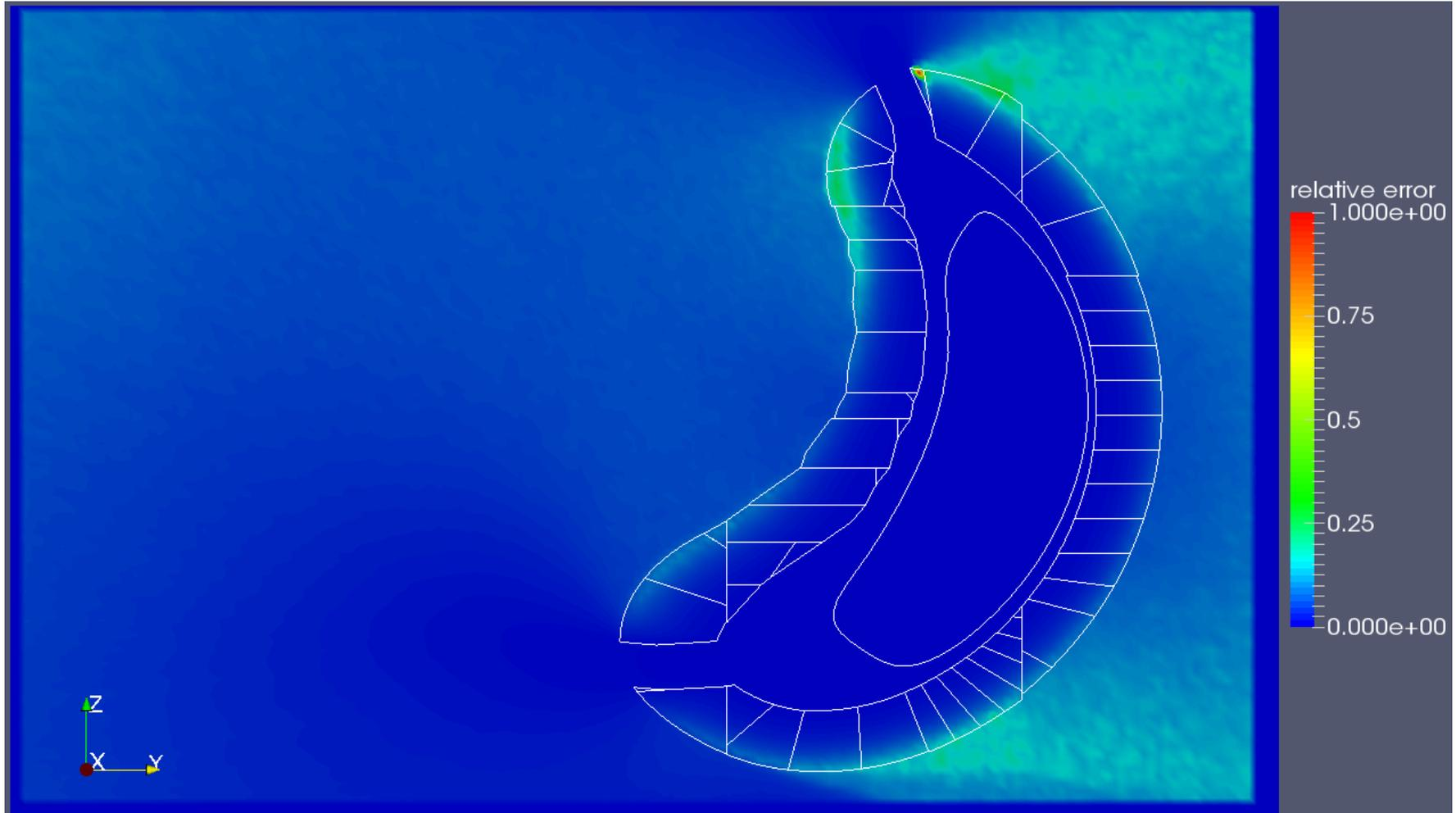
Error of the neutron flux meshtally in the perpendicular to the main axis; geometry and last closed flux surface are shown inside
