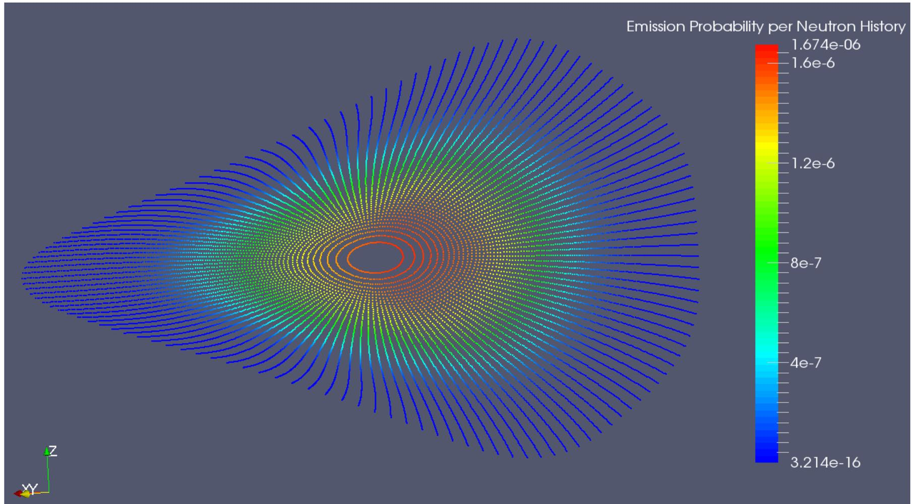
Emission probability of the source perpendicular to the main axis
