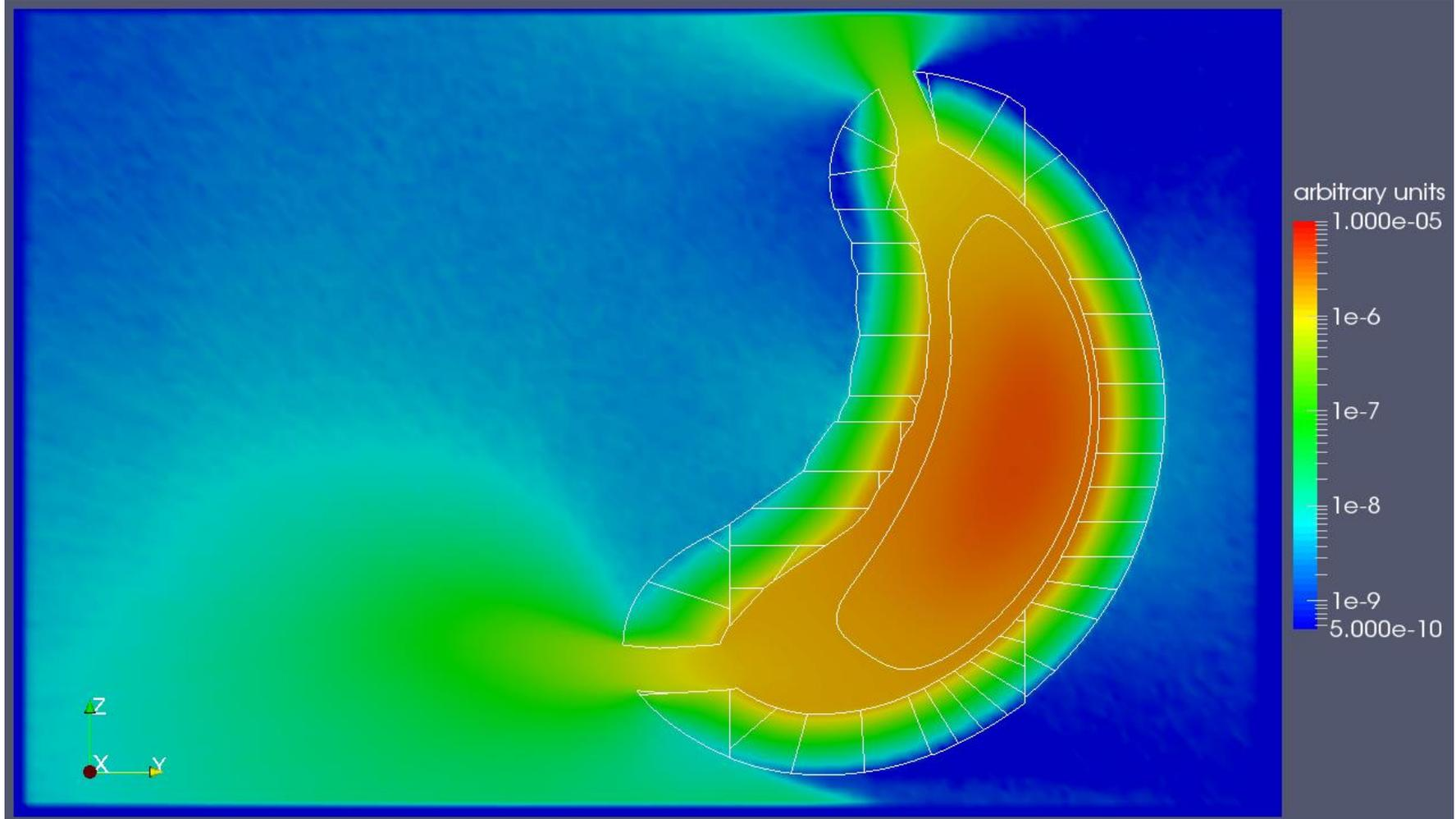
Result of the neutron flux distribution with arbitrary units in the perpendicular to the main axis; geometry and last closed flux surface are shown inside
