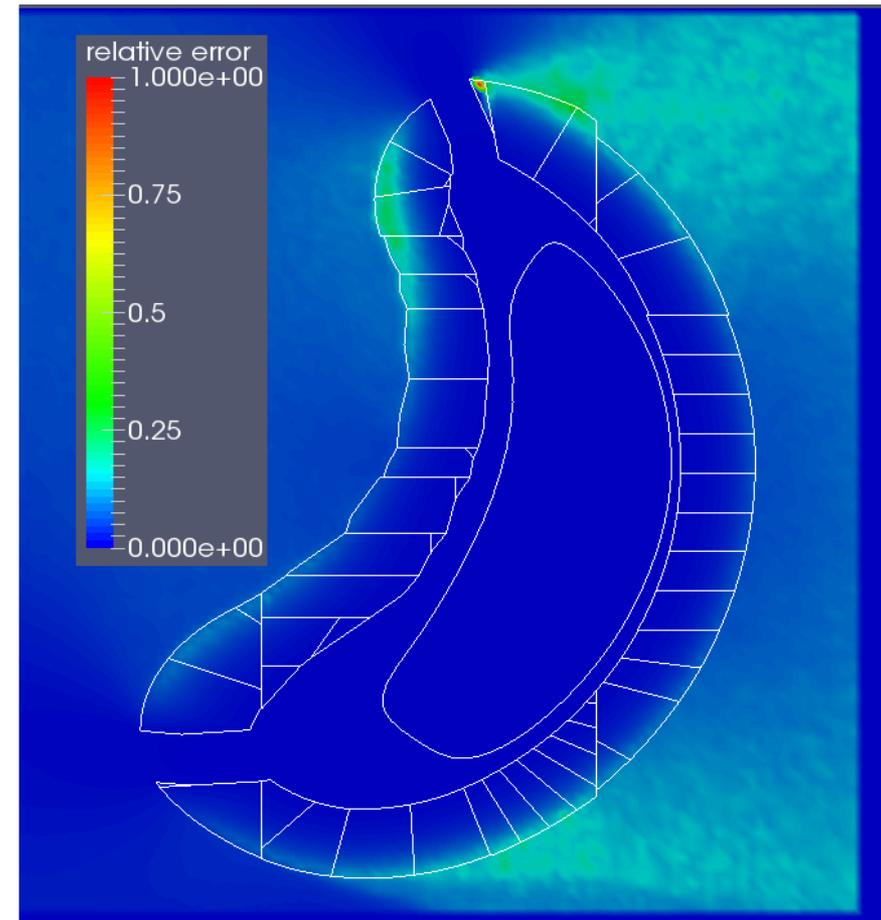
Distribution in plane perpendicular to the main axis. Geometry and last closed flux surface (white) is also shown.
