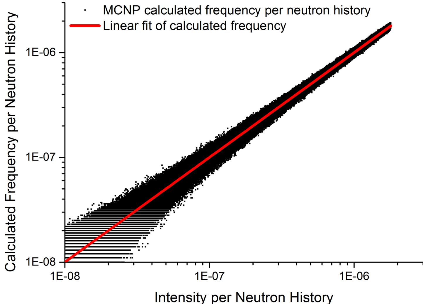
Calculated frequency of the source positions compared with the original intensity
