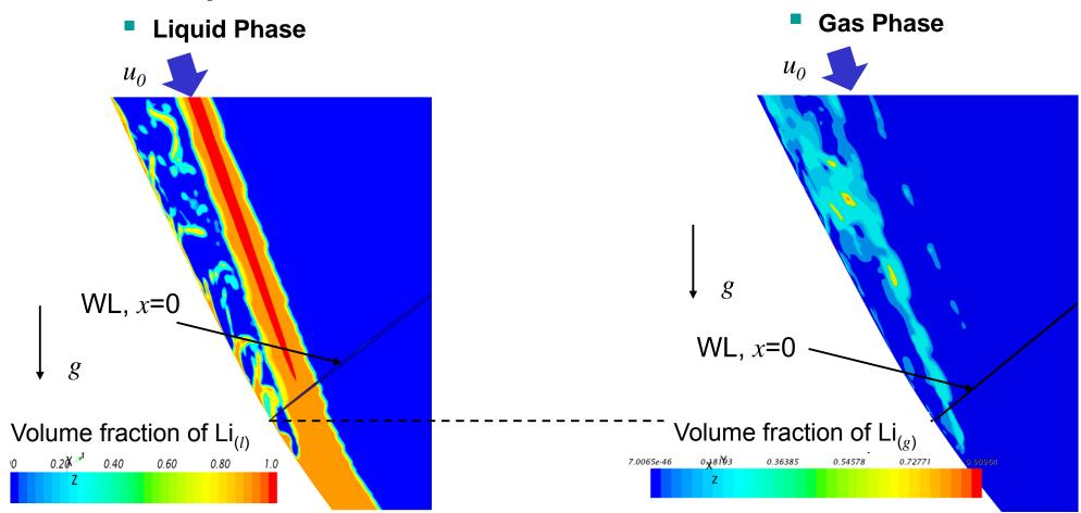
Interaction of impinging jet with reversed flow
