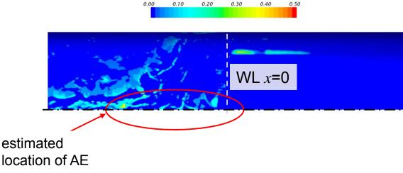
Static pressure on the pipe wall
