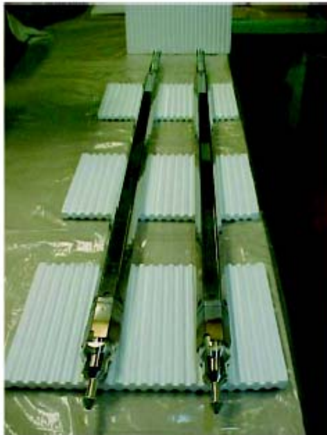
Fig. 12 Appearance of fabricated ODS fuel assemblies (BC358E and BC359E)
