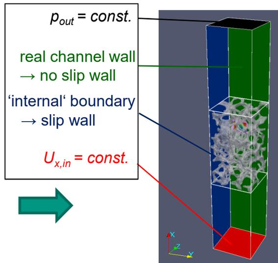
adapted CFD model set-up
