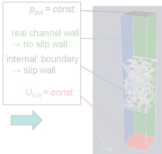
adapted CFD model set-up
