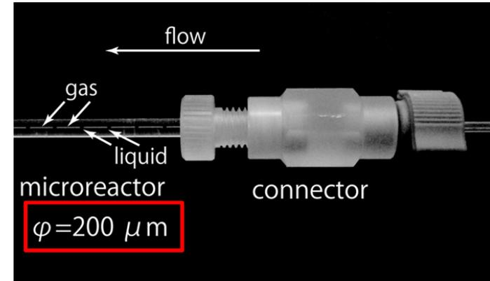
Microreactor for hydrogenation of nitrobenzene from Kataoka et al., Applied Catalysis: General 427-428 (2012) 119-124
