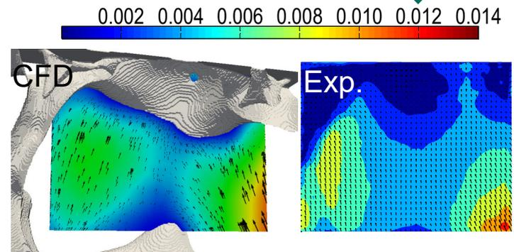
Comparison of calculated and measured local (time-averaged) velocity fields
