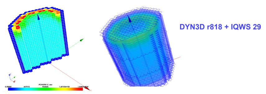
Power displaced to the top of the core in the axial layer 29 and 30.
