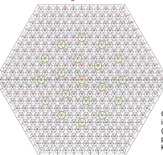
MESH DETAILS: 331 fuel rods 660 subchannels 876 gaps
