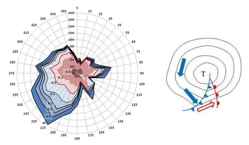
data: FINO1, 2005, wind direction at 80 m, stability at 60 m
