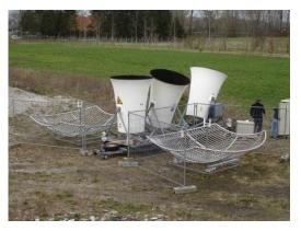
**Wind-LIDAR,** optical backscatter, Doppler analysis, wave length ~ 1.5  $\mu$ m  $\rightarrow$  wind and aerosol profiles
