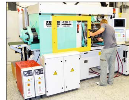
Injection molding of green parts
