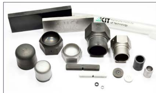
Green parts (dark), finished parts (brighth)
