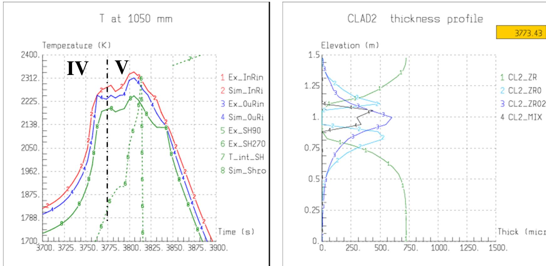
ASTEC predicts temperature escalation due to reflooding at 1050 mm
