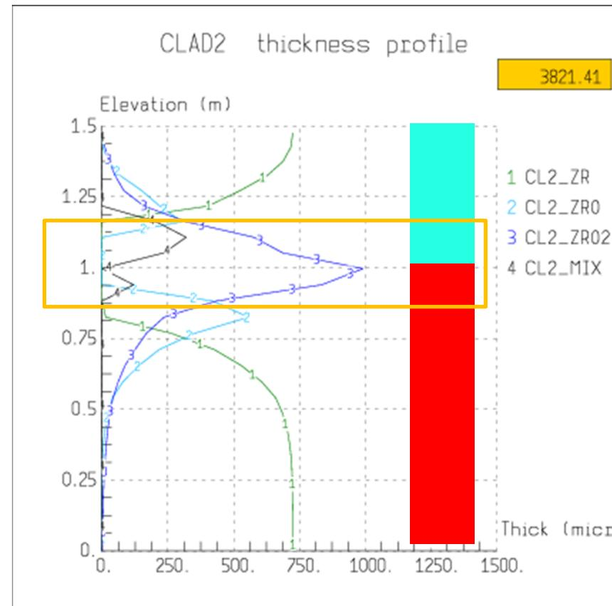
The upper part of the active zone and the lower part of the heated zone are further oxidized during re-flooding
