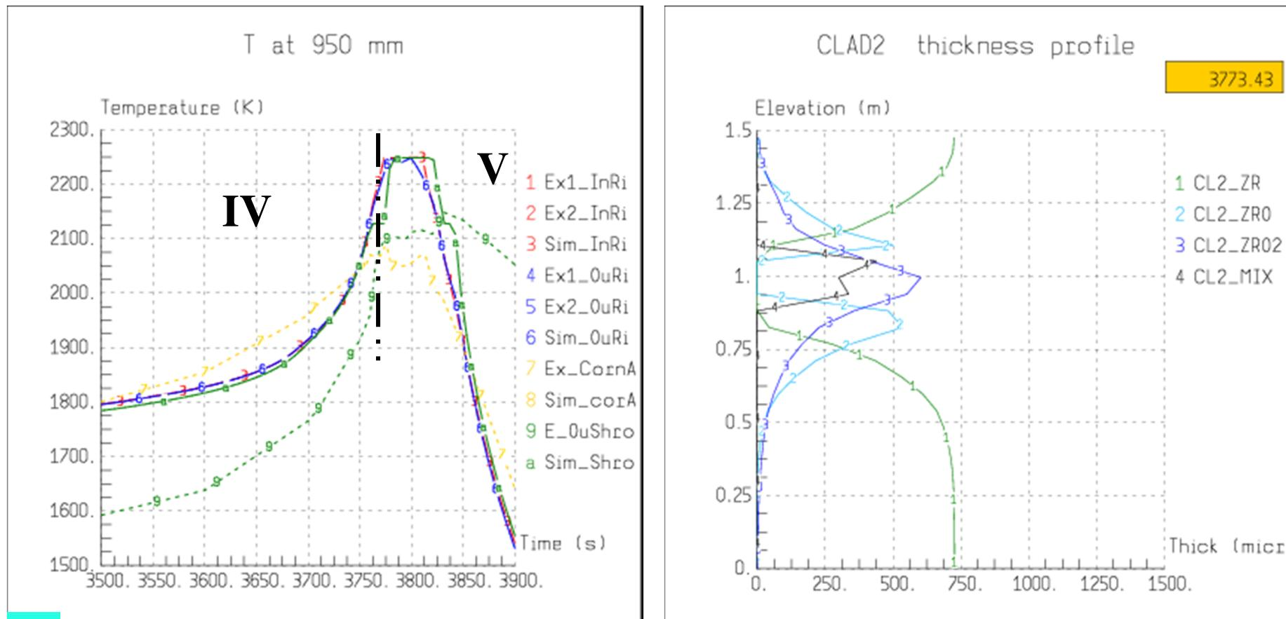
Predicted temperature escalation in fuel rod simulators shows a similar trend than experimental corner rod A
