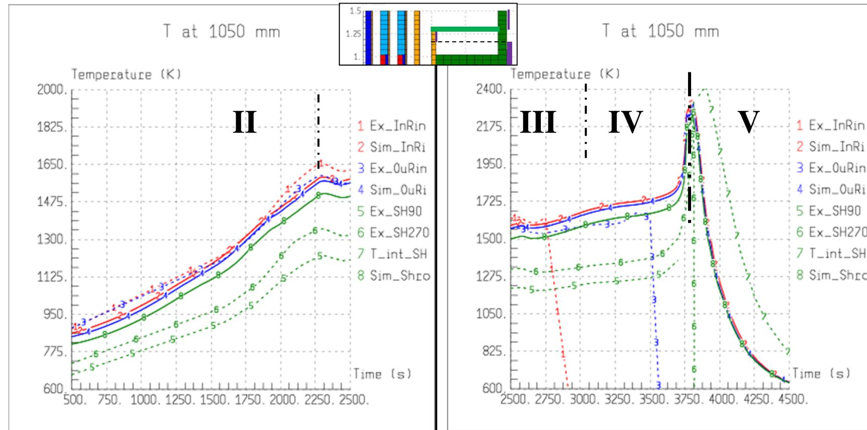
Temperature escalation occurred at 950 mm propagates upwards → T runaway
