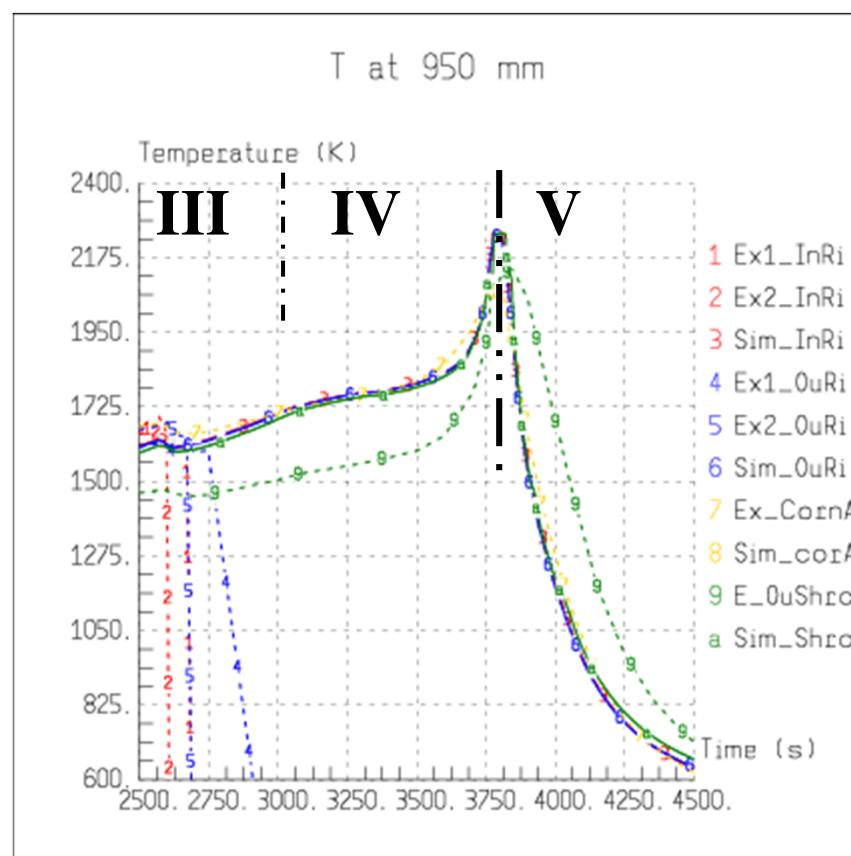
**Trends are very well predicted by ASTEC in fuel rod simulators until quenching
