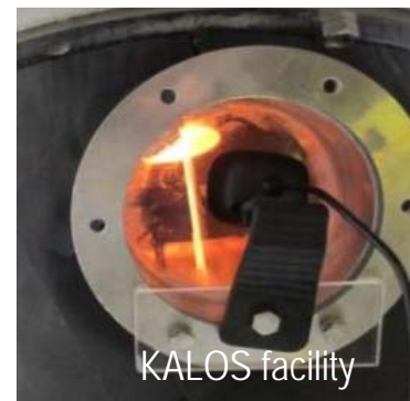
Fabrication and characterization of Li_4SiO_4 (with 10-20% Li_2TiO_3 )
