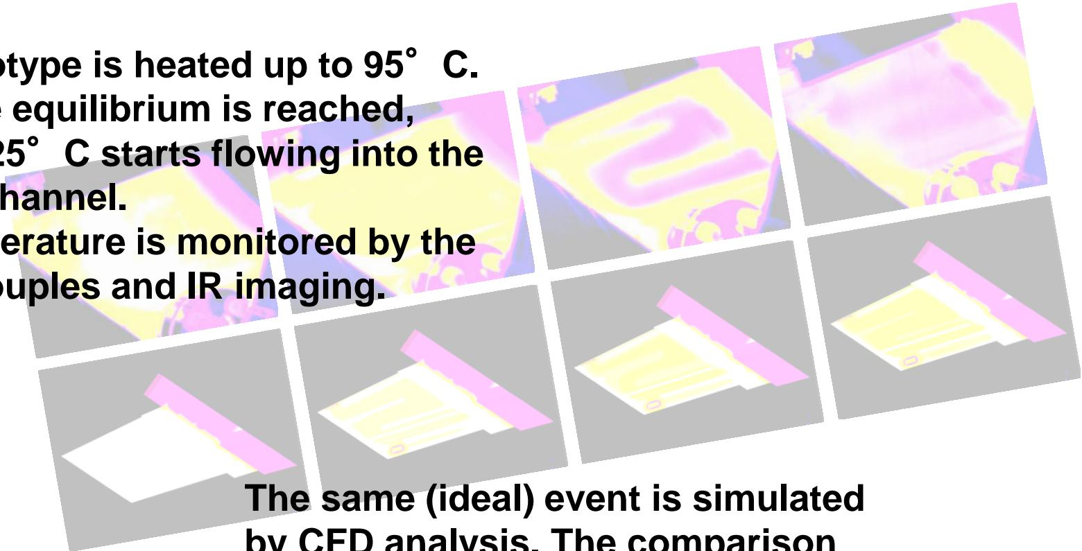
The same (ideal) event is simulated by CFD analysis. The comparison between the simulation and the experiment will provide information about the validity of the model.
