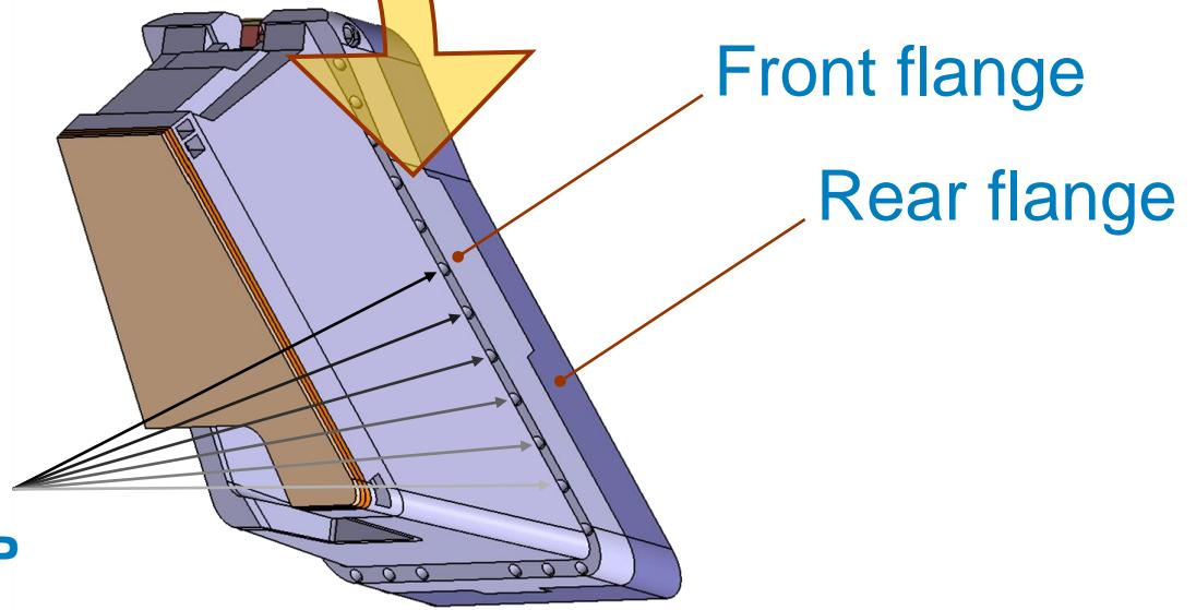
**Bolts are used to connect the Blanket Shield Module to the mainframe of the UPP**
