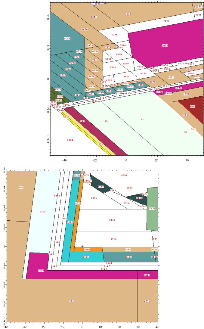
The model is divided into several sectors to take into account of the non-constant heat deposition in the steel and
