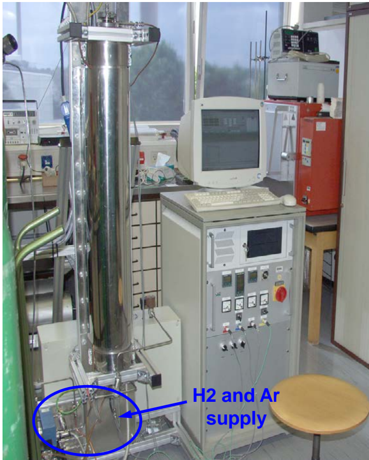
vertical 3-zones tube furnace LORA (height 60 cm)
