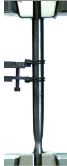
ductile not hydrogenated sample with pronounced contraction
