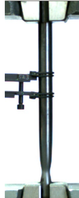
ductile not hydrogenated sample with pronounced contraction
