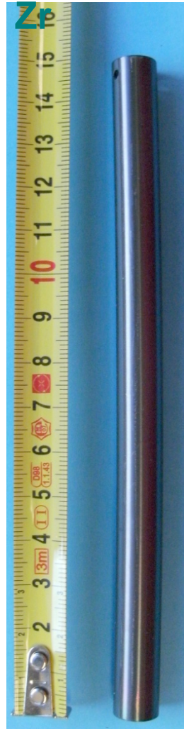
H19Z4: annealed at 800^\circ\text{C} with \text{H}_2 (37 mbar); \Delta t = 240 s \Delta m_{\text{H}} = 1600 wppm
