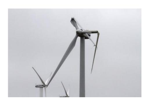
This turbine has been damaged by gale force winds in Northern Germany in February 2011
