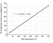
■ The outgassing rate of a surface is temperature dependent. The samples are placed at the midpoint of the oven. A temperature calibration was carried out before starting the sample outgassing measurements.
