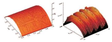
The outgassing rate depends on the surface finish of the material. Its effect can be observed only using the real area of the samples in the outgassing calculations. Roughness measurements were performed in order to calculate the surface factor  $f_{z} = A_{z}/A_{y}$  of each sample.
