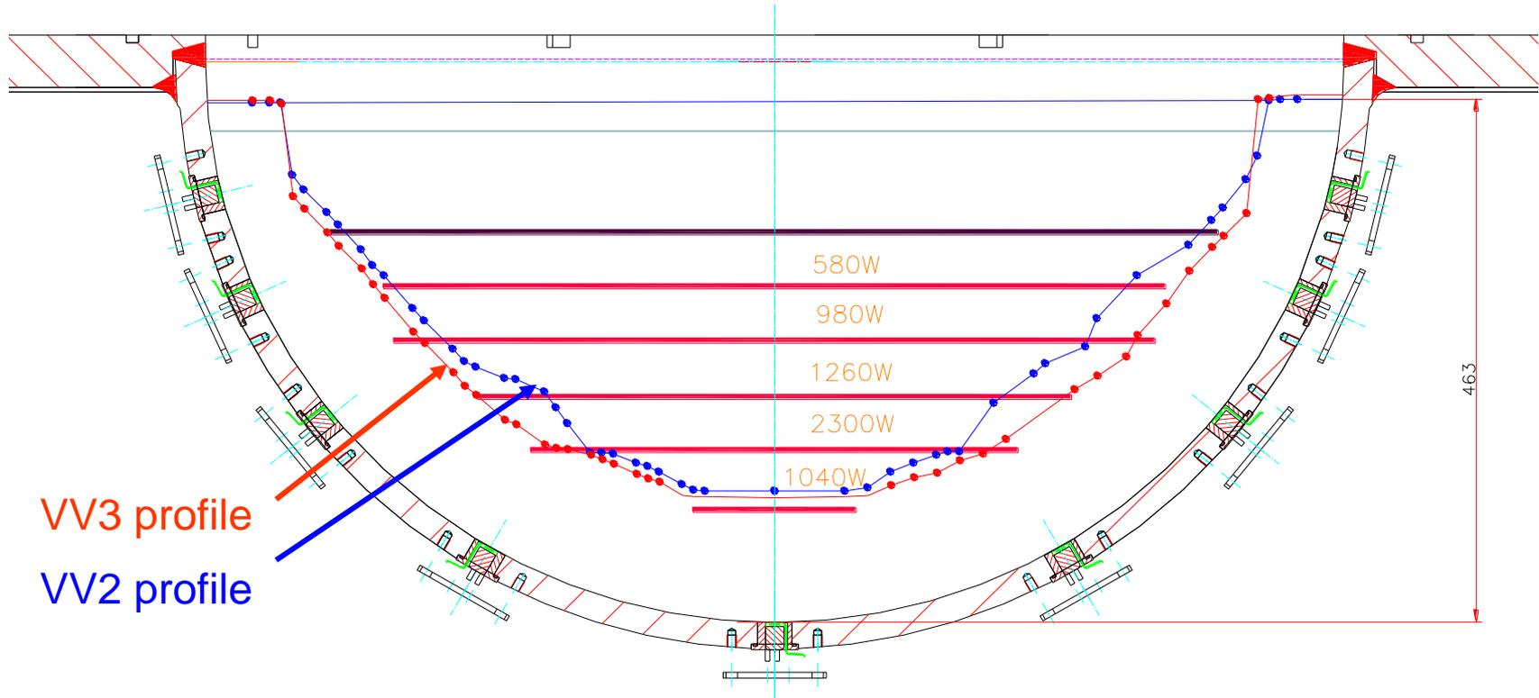
Total heating power: 6200W, heterogeneous heating
