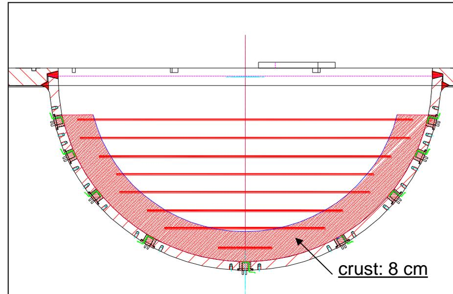
desired crust profile in the LIVE-CERAM: thick and uniformly
