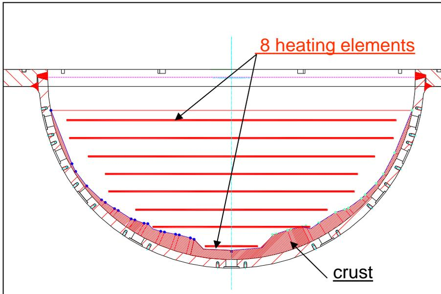
crust profile in a volumetrically heated pool: thin and non-uniformly
