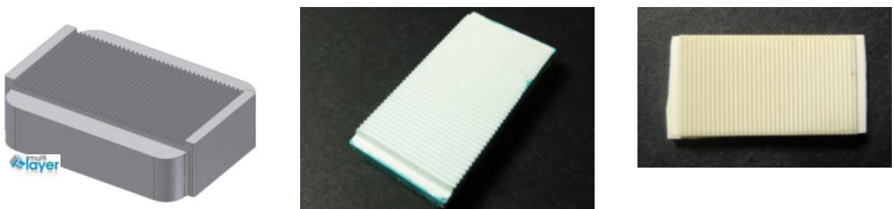
Figs. 6-8: A test mould insert used for the development of IML-MicroPIM, height of the zig-zag structure is approx. 550\mu\text{m} (left); green body after tape insertion, feedstock injection, and demoulding (middle); sintered part, height of the zig-zag structure now is approx. \mu\text{m} (right).
