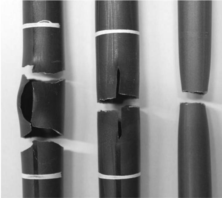
Rupture near to the burst opening due to hydrogen enrichment
