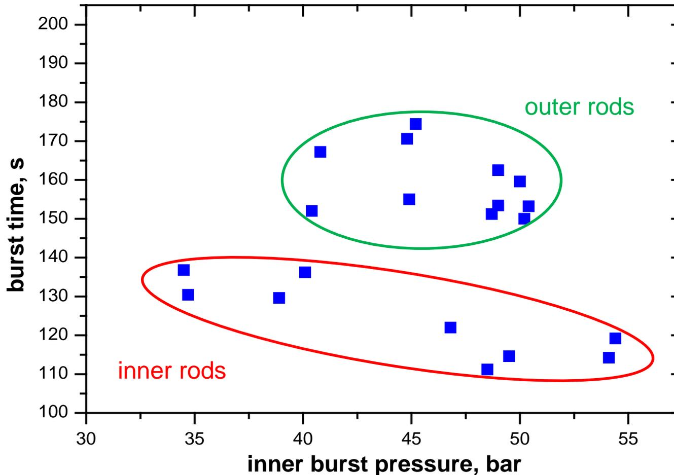
Only slightly effect of inner pressure on the burst time
