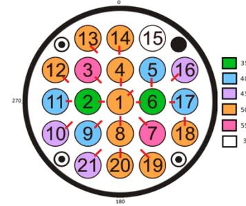
Cross section according 16 x 16 KONVOI geometry
