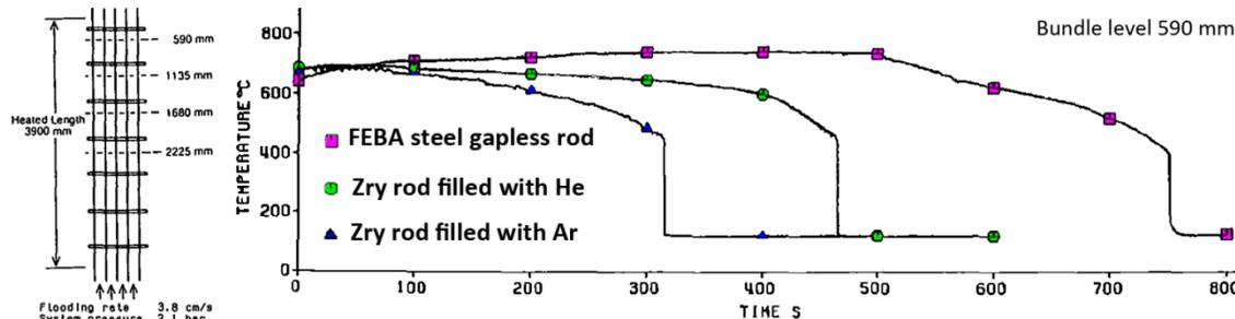
**Peak cladding temperatures and quench times of SEFLEX (Zry) and FEBA (SS) bundles**
