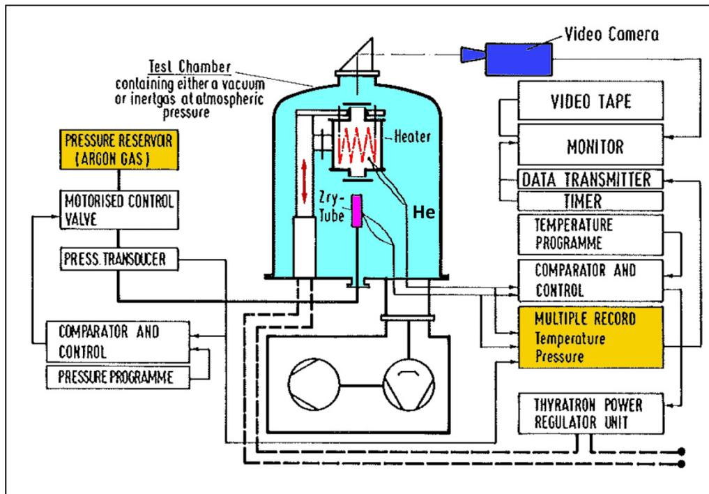
scheme of **TUBA** rig (TUBE Burst Apparatus)
