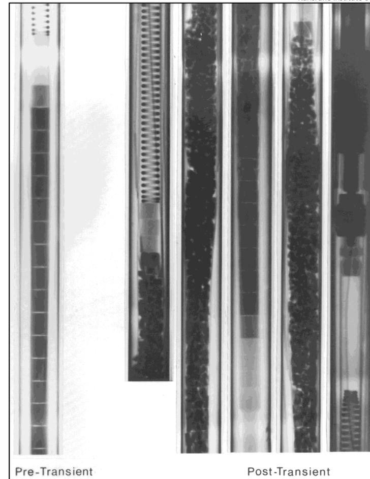
**neutron radiography: lost of shape of fragmented pellets after ballooning (rod F1, burnup 20 GWd/tU)**
