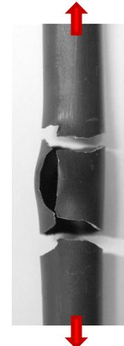
double ruptures due to hydrogen embrittlement ( $C_H < 1000 \text{ wppm}$ )
