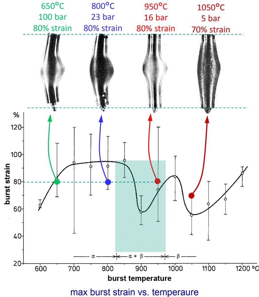
1) two minimums of the burst strain: at 900°C ( $\alpha + \beta$  region) and 1050°C ( $\beta$  region);
