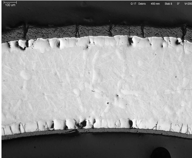
450 mm: outer ZrO<sub>2</sub> 75 µm, inner ZrO<sub>2</sub> 25 µm, α-Zr(O) 70 µm (outer and inner), prior β-Zr rest
