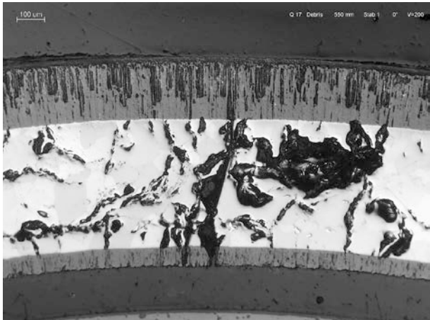
rod #1 (similar to #2 - #6): outer \text{ZrO}_2 220 \mu\text{m} ; inner \text{ZrO}_2 70 \mu\text{m} ; through-going crack
