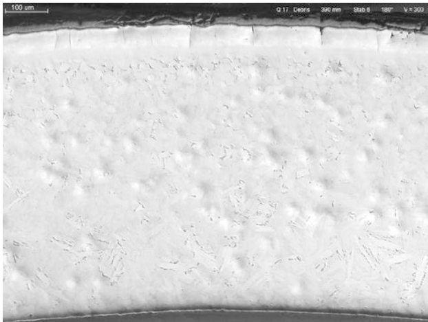
rod #6: outer \text{ZrO}_2 25 \mu\text{m} ; \alpha\text{-Zr(O)} 50 \mu\text{m} ; no debris \rightarrow good heat removal
