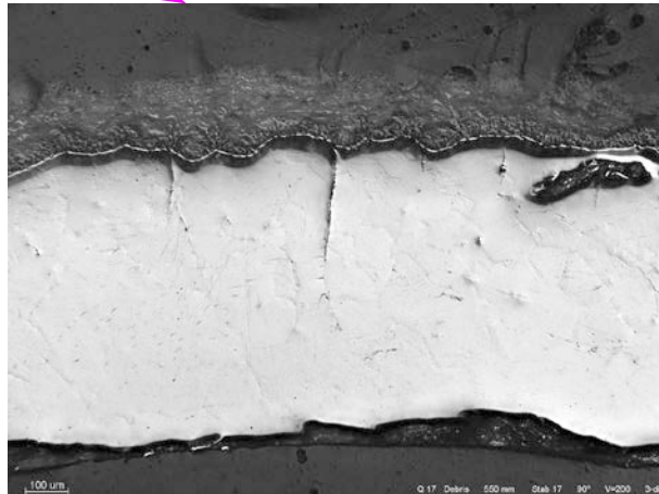
rod #17: outer \text{HfO}_2 160 \mu\text{m} , breakaway \alpha\text{-Hf(O)} remnant
