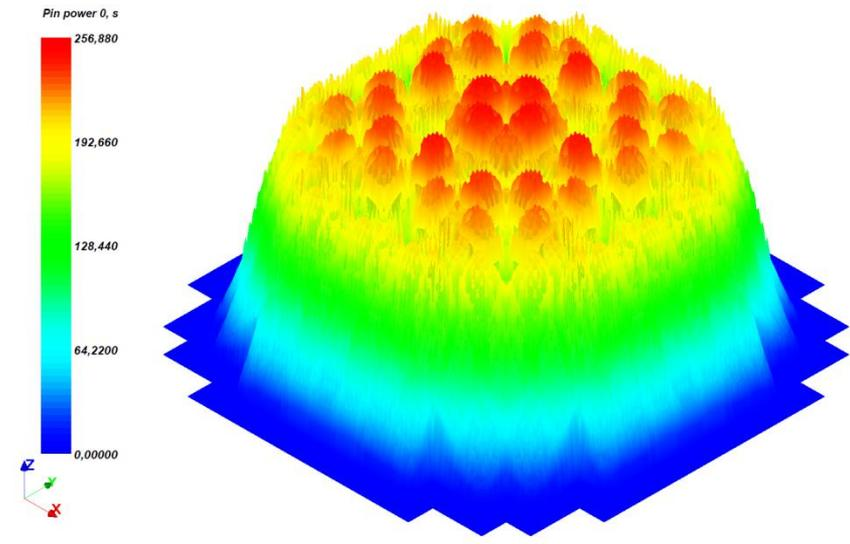
**Fuel pin / sub-channel resolution coupled NK
