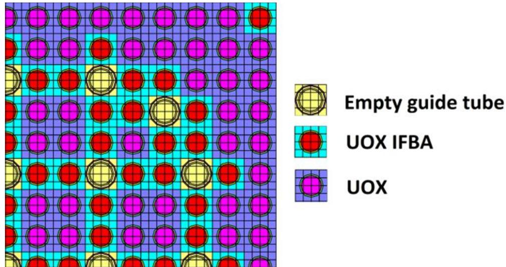
Fig. 2. Composition of a Quarter of a 17x17-25 UOX Fuel Assembly
