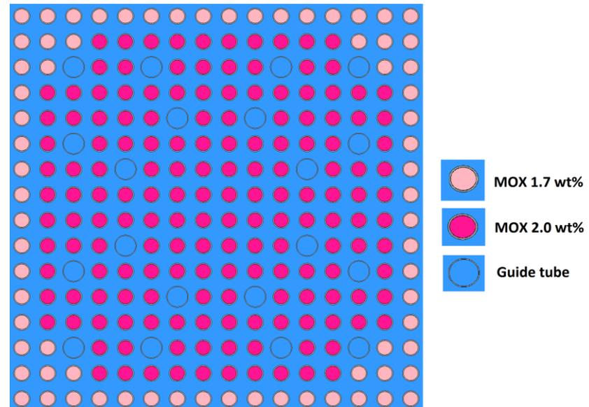
Fig. 1. Composition of a 16x16-25 MOX Fuel Assembly
