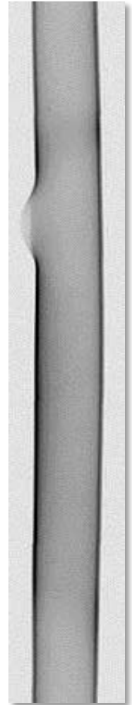
rod #5: neutron radiography
