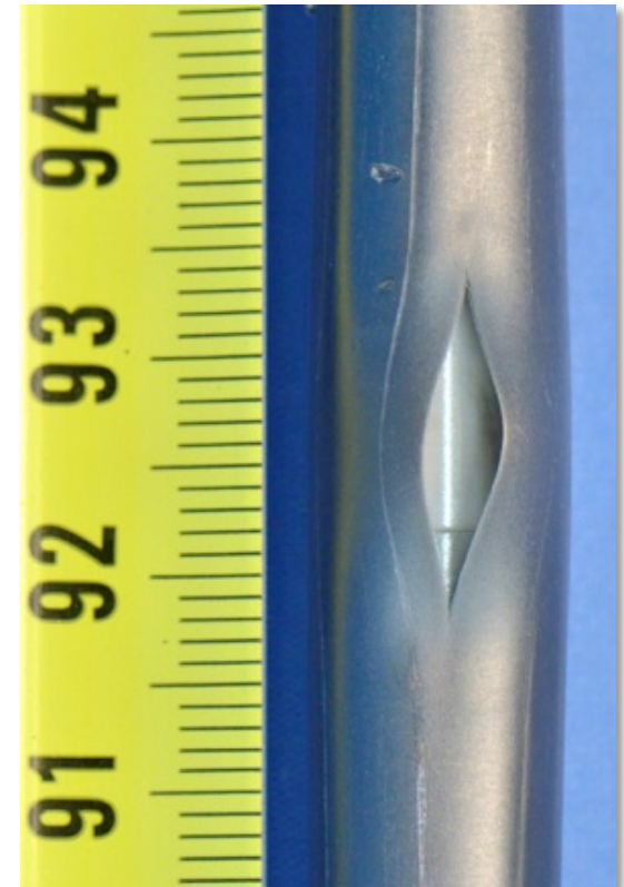
rod #7: burst opening
