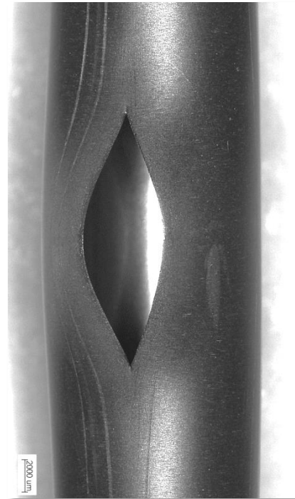
rod #16: burst opening
