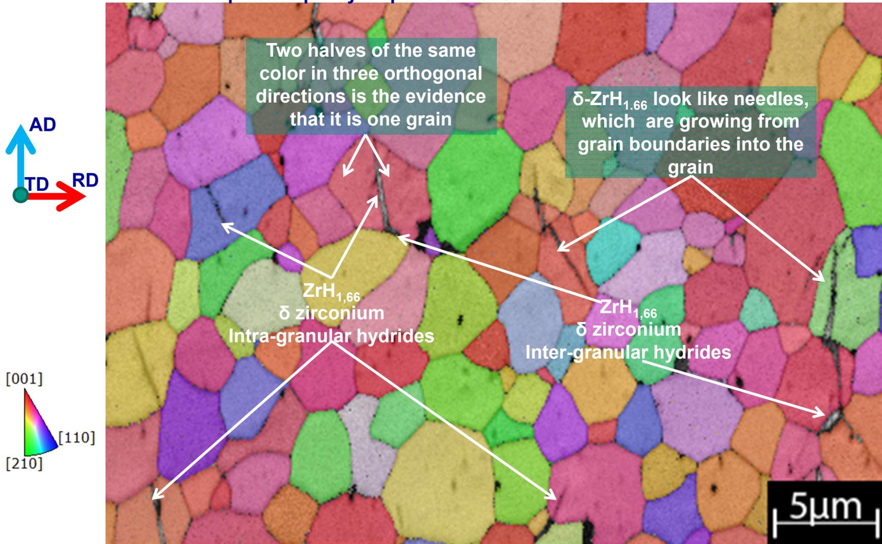
99.3% Zr, 0.7% ZrH<sub>1.66</sub>,  $\gamma$ -ZrH – not detected (on the basis of image analysis)
