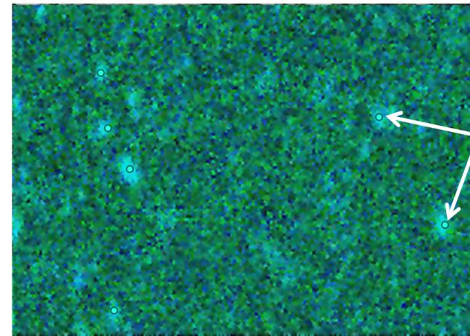
EDX-analysis of intermetallic particles distribution (Fe + Cr) mostly near to grain boundaries
