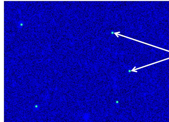
EDX-analysis of impurities distribution (Fe) near to grain boundaries and inside the grains
