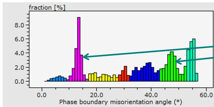
There is also another accommodation mechanism on the grain boundaries of Zircaloy-4 – low angle from one side and high angle boundary on the other side of hydride together give  $\sim 60^\circ$  which is a characteristic direction for hexagonal lattice
