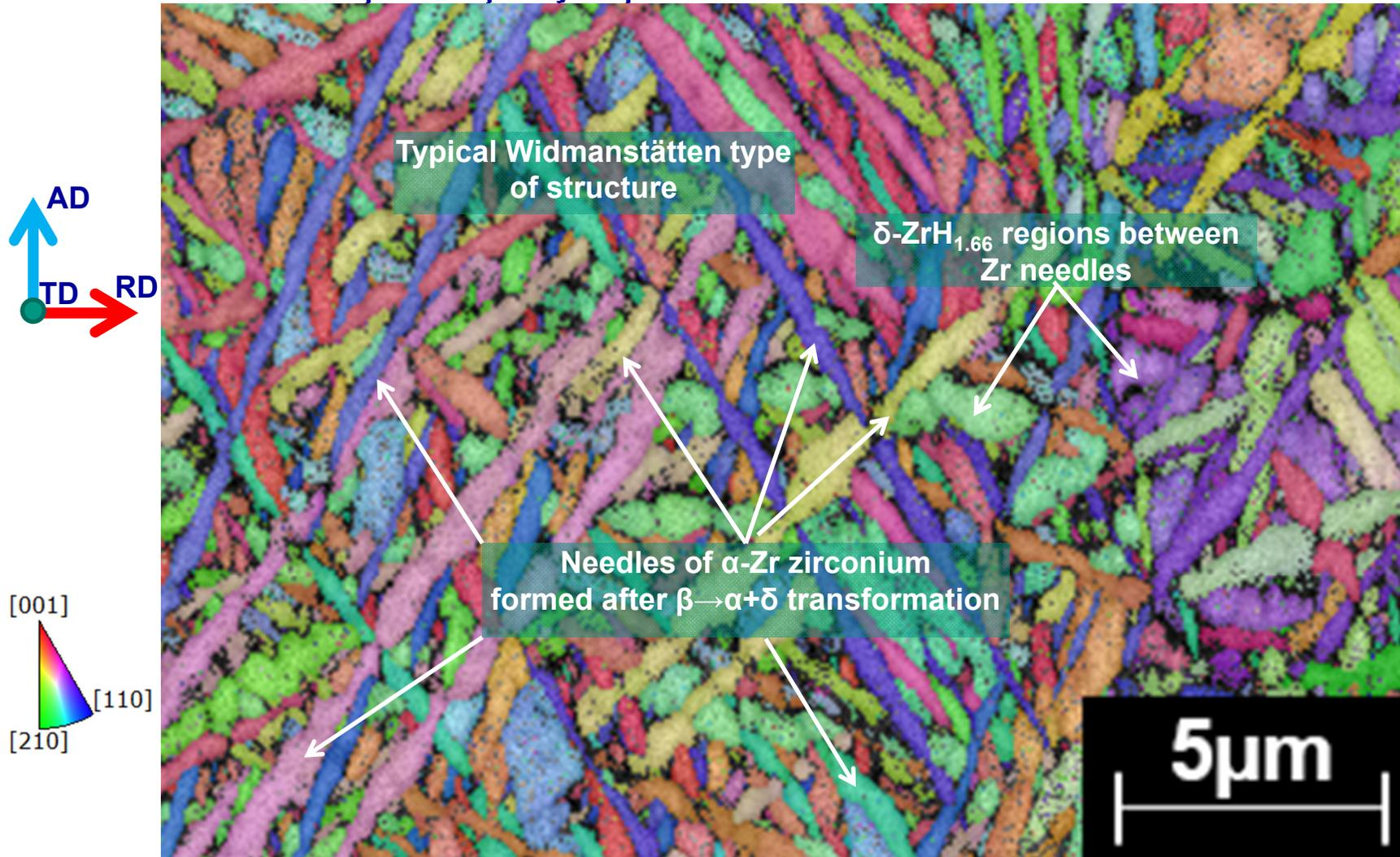
60% Zr, 39%  $\delta\text{-ZrH}_{1.66}$ , 1%  $\gamma\text{-ZrH}$  (on the basis of image analysis)
