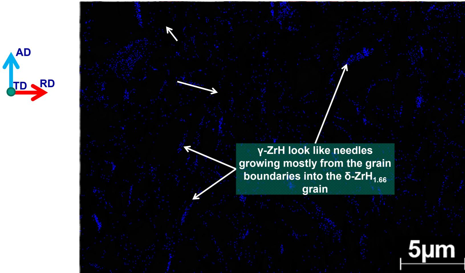
27.1% Zr, 70.6%  $\delta$ -ZrH<sub>1.66</sub>, 2.35%  $\gamma$ -ZrH (on the basis of image analysis)
