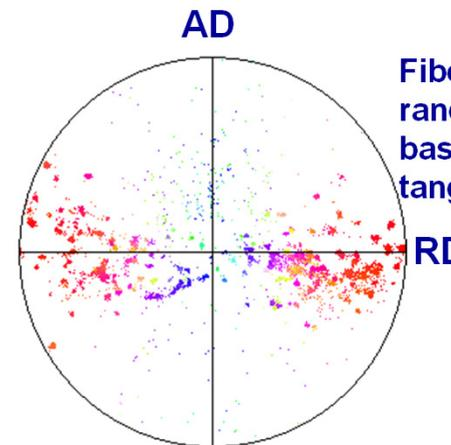
Fiber texture with a random distribution of basal poles in the radial-tangential plane\*
