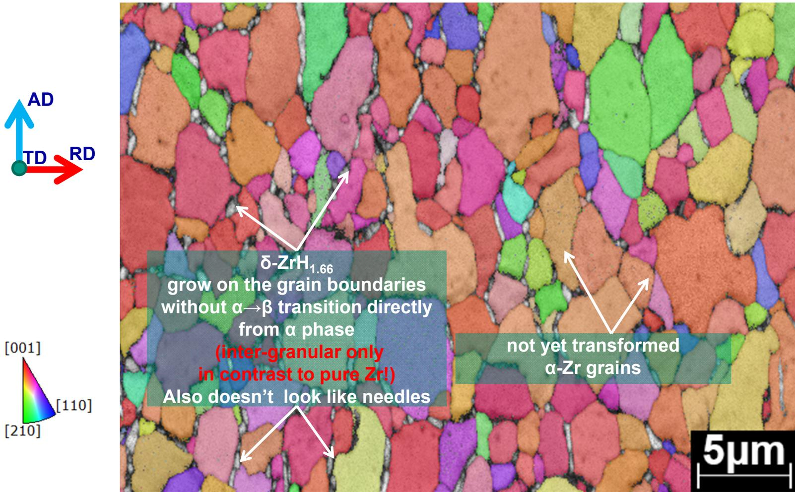
94.8% Zr, 5.2%  $\delta$ -ZrH<sub>1.66</sub>,  $\gamma$ -ZrH – not detected (on the basis of image analysis)
