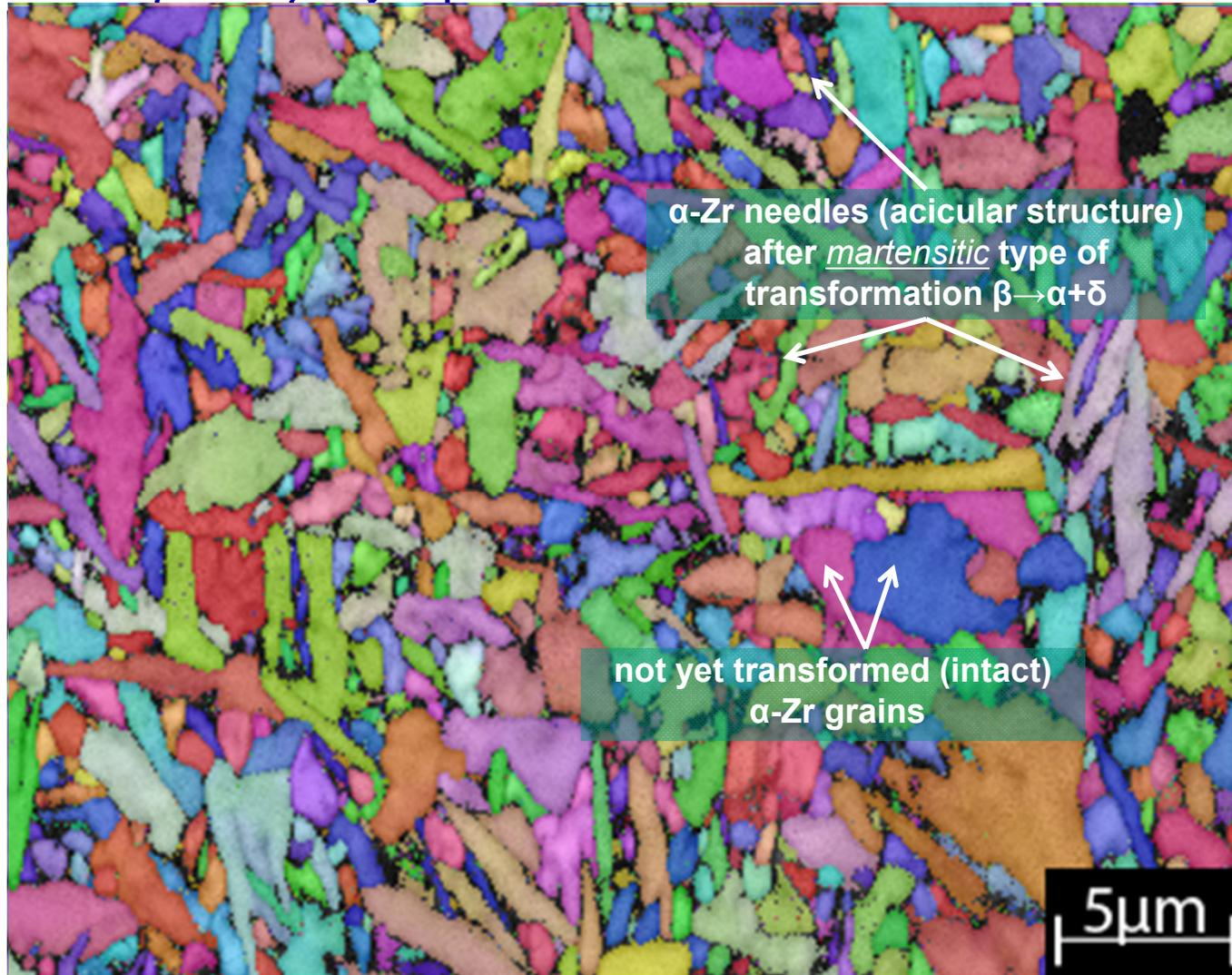
72.6% Zr, 26.5%  $\delta$ -ZrH<sub>1.66</sub>, 0.8%  $\gamma$ -ZrH (on the basis of image analysis)
