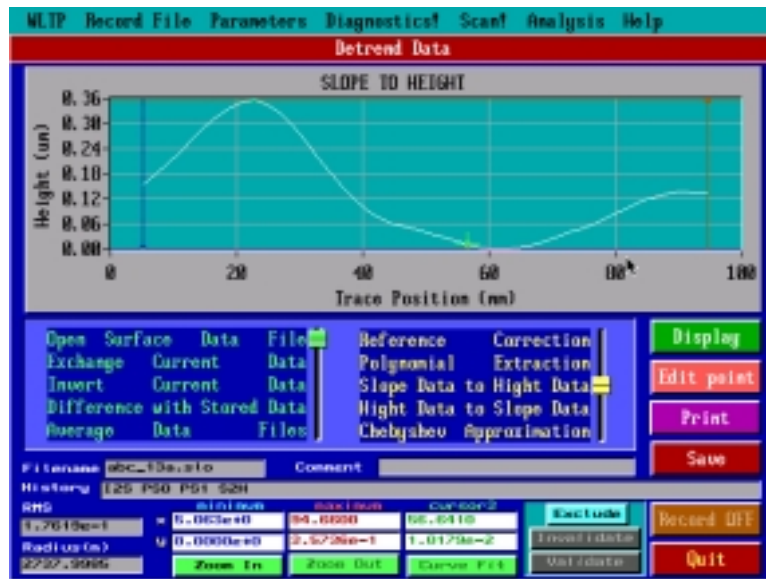
Figure 34. The height data versus trace position of the vertical focusing mirror with a rms slope error \sigma_{\text{Slope},v} = 9.5 \mu\text{rad} .
