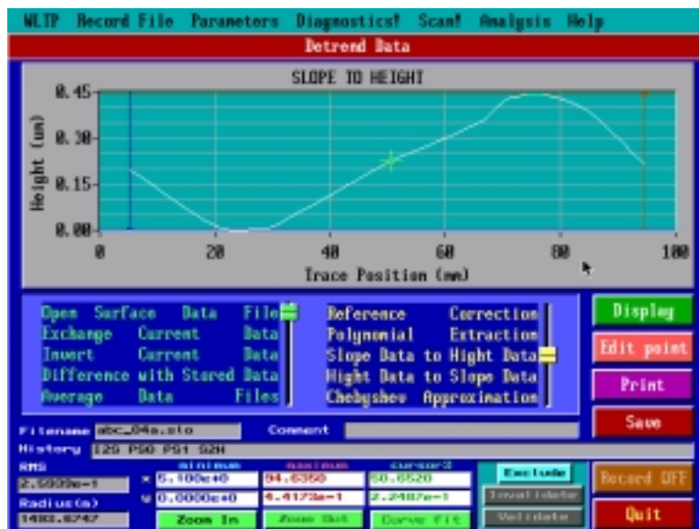
Figure 35. The height data versus trace position of the horizontal focusing mirror with a rms slope error \sigma_{\text{Slope},h} = 10.7 \mu\text{rad}
