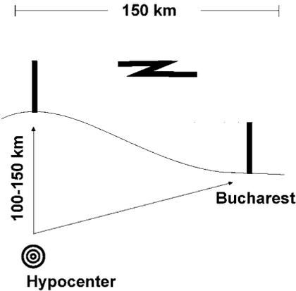
Figure 8: Sketch of the early warning system for Bucharest that will provide about 25 s warning time based on traveltime differences between S- and P-waves
