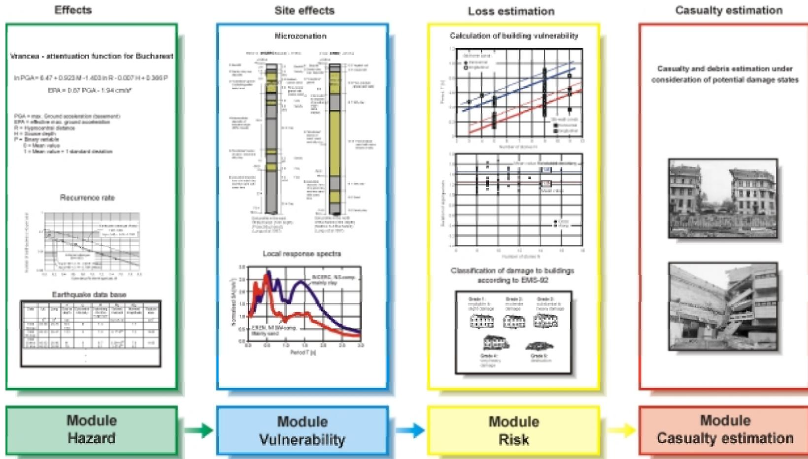
Figure 6: Scheme for modules of the damage and loss estimation tool (after Lungu and Coman [6] and Lungu et al. [7])
