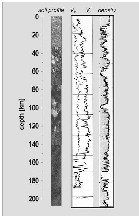
Figure 5: Illustration of soil profile with S- and P-wave velocities and density log
