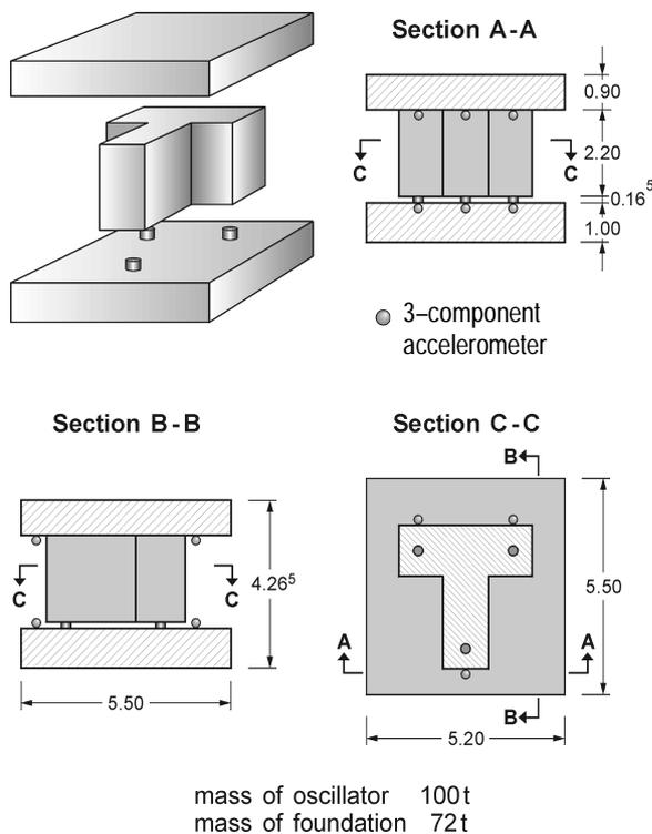
Figure 3: Design of the Test Building of the Multidisciplinary Seismic Test Site
