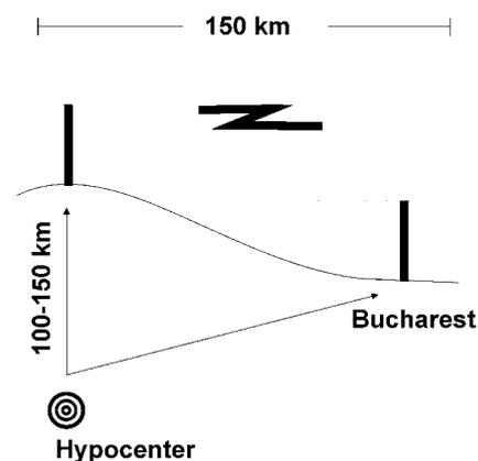
Figure 8: Sketch of the early warning system for Bucharest that will provide about 25 s warning time based on traveltime differences between S- and P-waves
