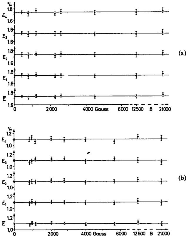
Fig. 2. The polarization effect  $E$  as a function of the target magnetization  $B$ .  $E_1$  to  $E_4$  belong to different combinations of the directions of the target and analyser magnetization, respectively. (a) pulse heights corresponding to a primary  $\gamma$ -energy of 660 keV. (b) a  $\gamma$ -energy of 470 keV.  $E$  is the average polarization effect.
