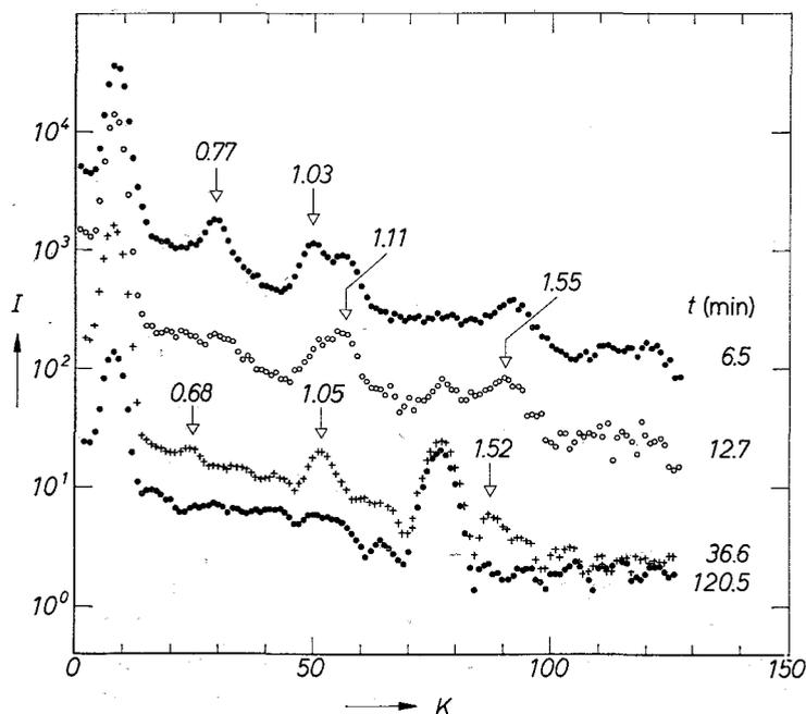
Fig. 3. Gamma spectra of a europium sample separated from a target irradiated with 40 MeV deuterons. The times shown represent the mean counting time after the end of bombardment. The numbers given in the figure show the energy of the different gamma peaks obtained in the analysis of the spectra. The peak at 0.68 MeV appears to be the sum-peak always observed in presence of annihilation radiation
