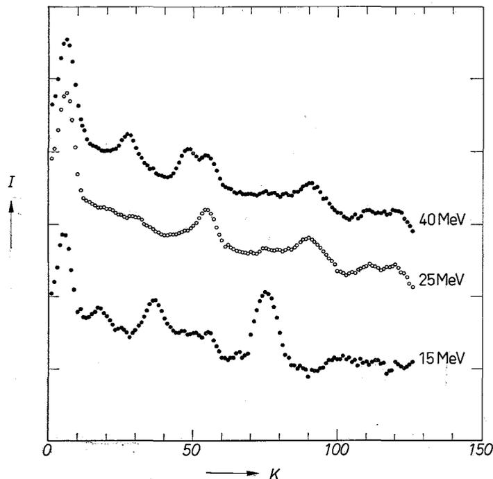
Fig. 2. Gamma spectra of europium samples recorded immediately after chemical separation from targets irradiated with 15, 25, and 40 MeV deuterons. The intensity  $I$  is plotted in arbitrary logarithmic units. The abscissa  $K$  represents channel number
