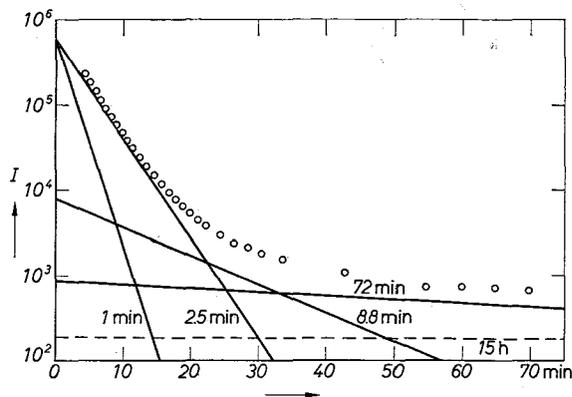
Fig. 5. Beta decay curve of a europium sample separated from a target irradiated with 40 MeV deuterons. The curve was measured with an Al-Absorber of 1080 mg/cm<sup>2</sup>
