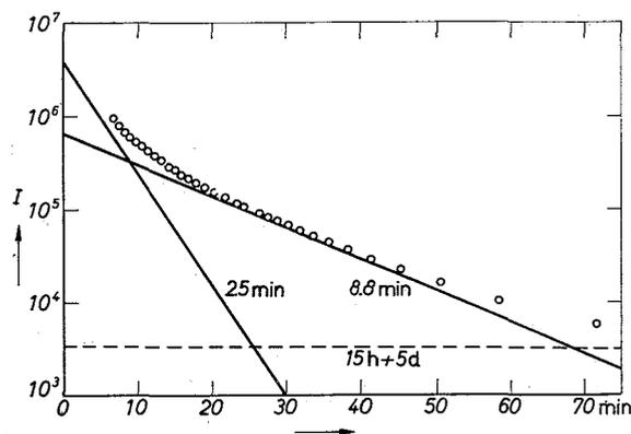
Fig. 4. Beta decay curve of a europium sample separated from a target irradiated with 25 MeV deuterons
