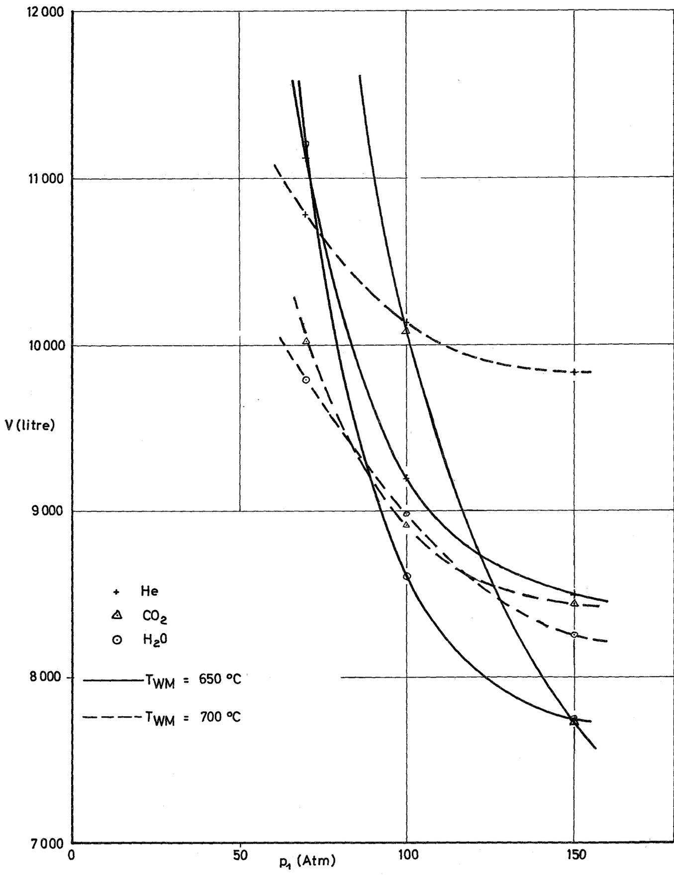
FIG. 5 CORE VOLUME FOR A CONSTANT NETT ELECTRICAL OUTPUT OF 1000 MWe .
