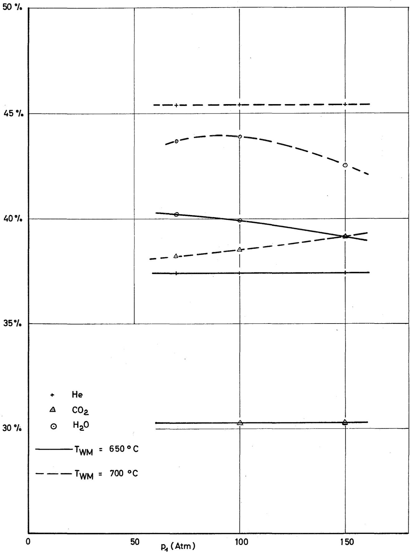
FIG. 6 CORE COOLANT FRACTION FOR A CONSTANT NETT ELECTRICAL OUTPUT OF 1000 MWe.
