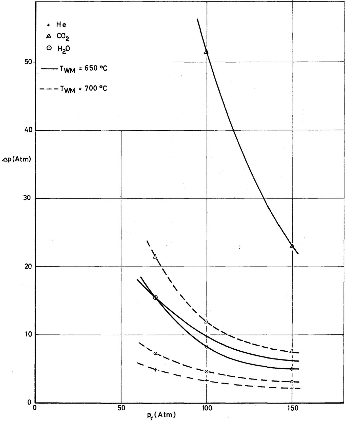
FIG. 2 PRESSURE DROP ACROSS THE CORE FOR A CONSTANT NETT ELECTRICAL OUTPUT OF 1000 MWe.
