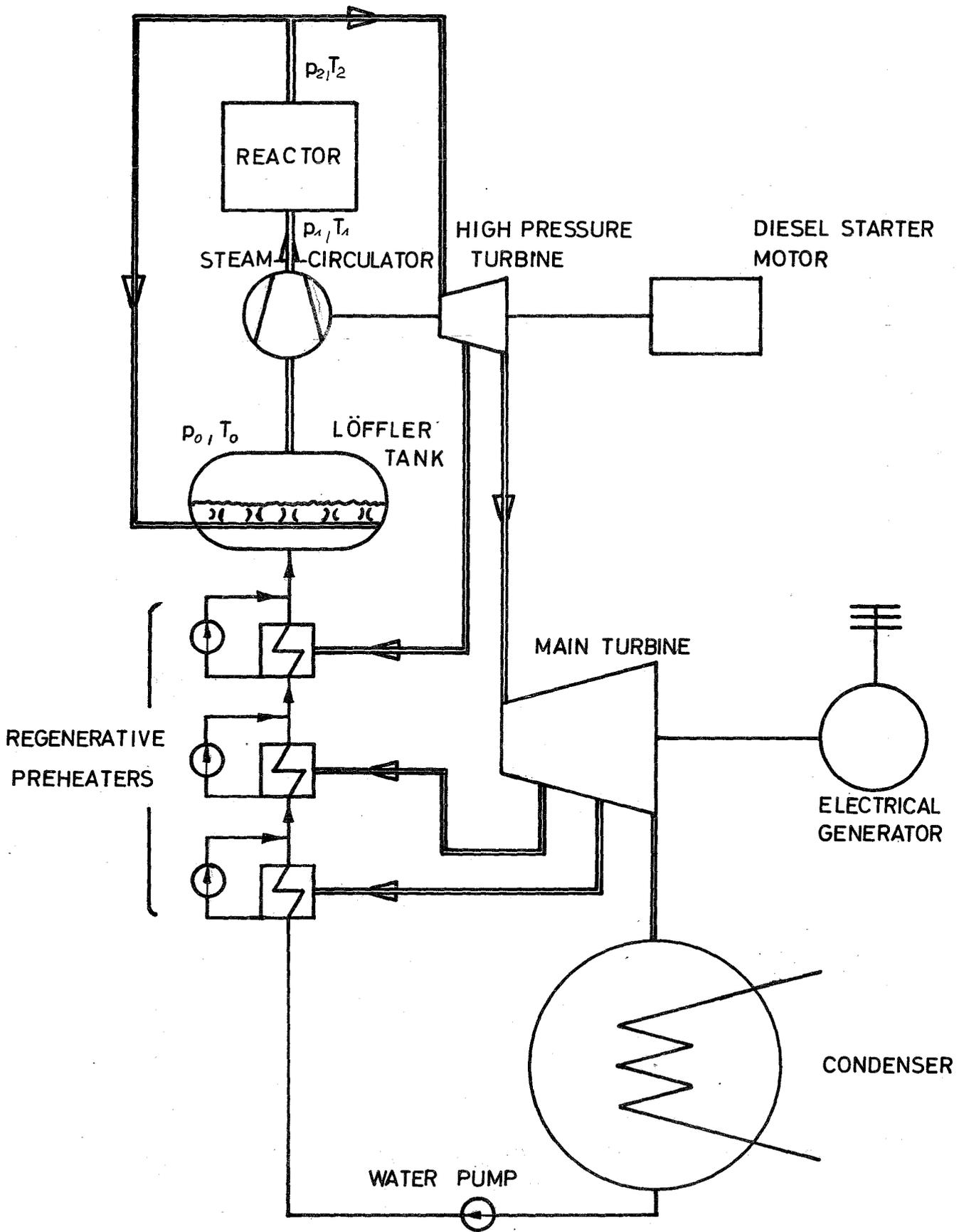
FIG. 1 SCHEMATIC FLOW DIAGRAM OF STEAM COOLED POWER PLANT
