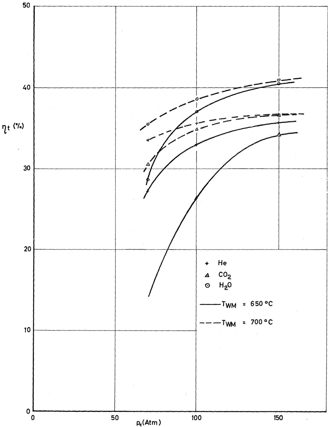
FIG. 3 NETT ELECTRICAL EFFICIENCY FOR A CONSTANT NETT ELECTRICAL OUTPUT OF 1000 MWe.
