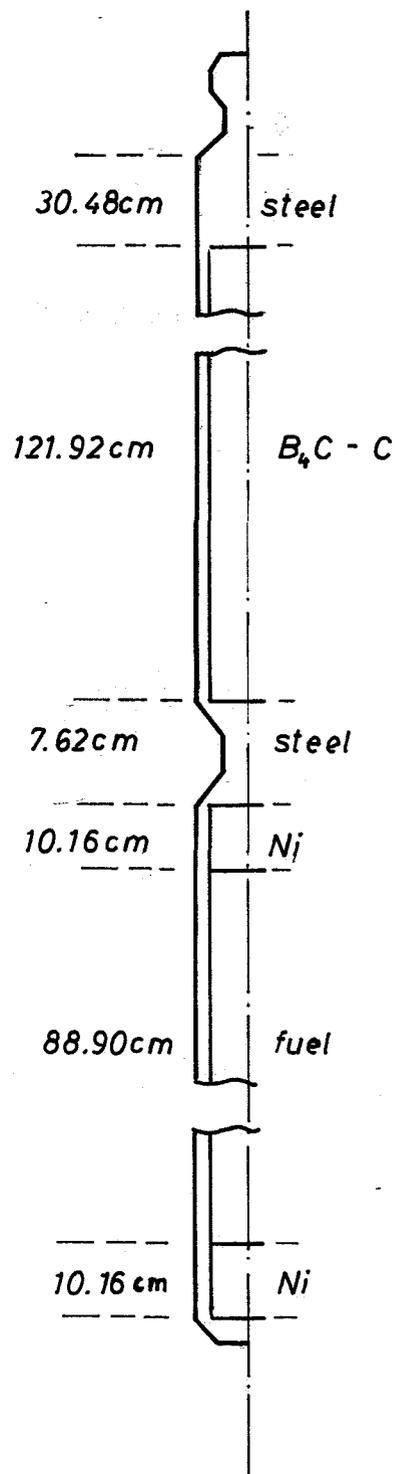
Fuel rod - Schematic diagram
