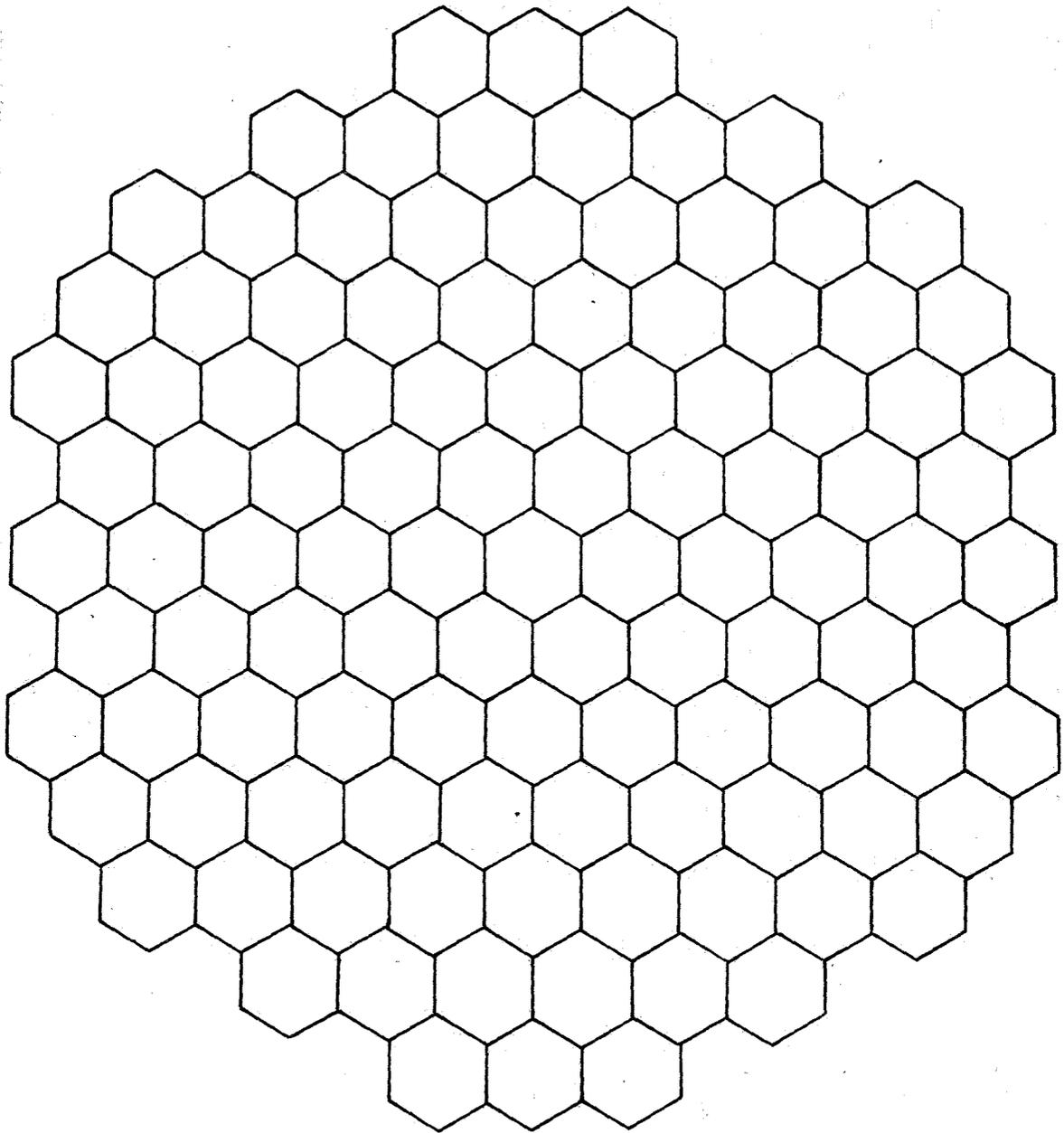
*Arrangement of core hexagonal channels*
