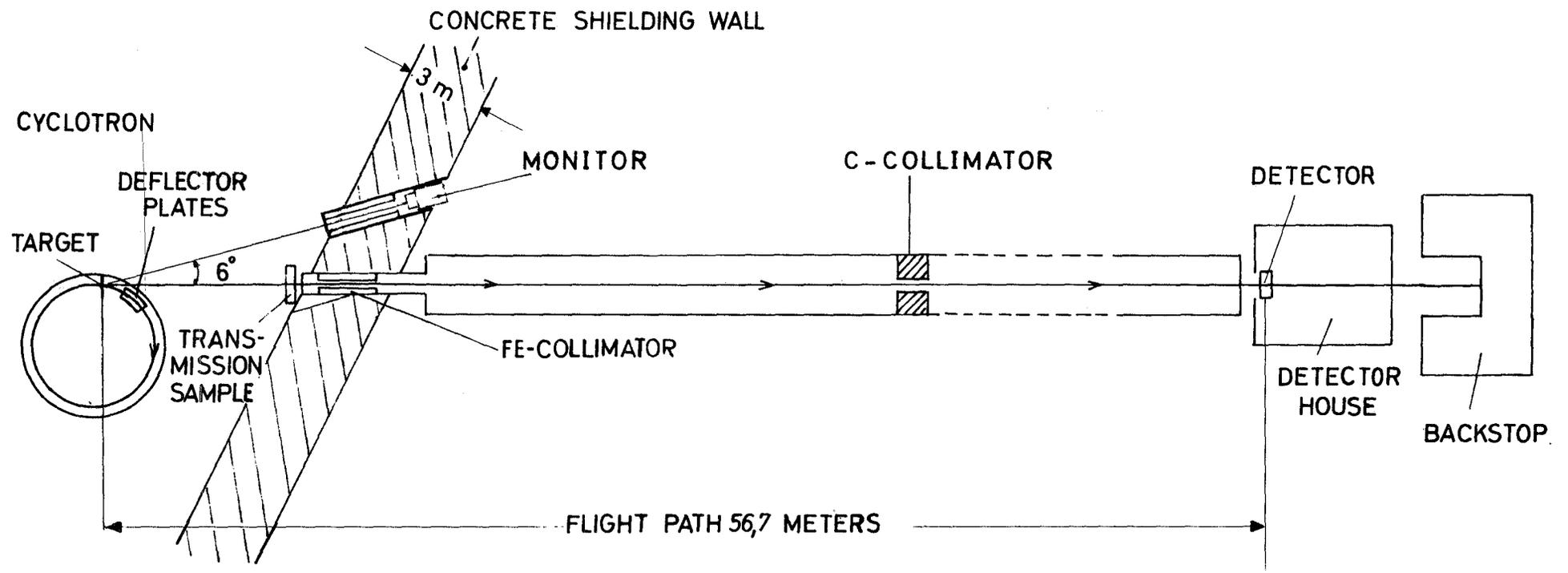
Fig.1: Geometry of the Karlsruhe isochronous cyclotron neutron time-of-flight spectrometer (top view).
