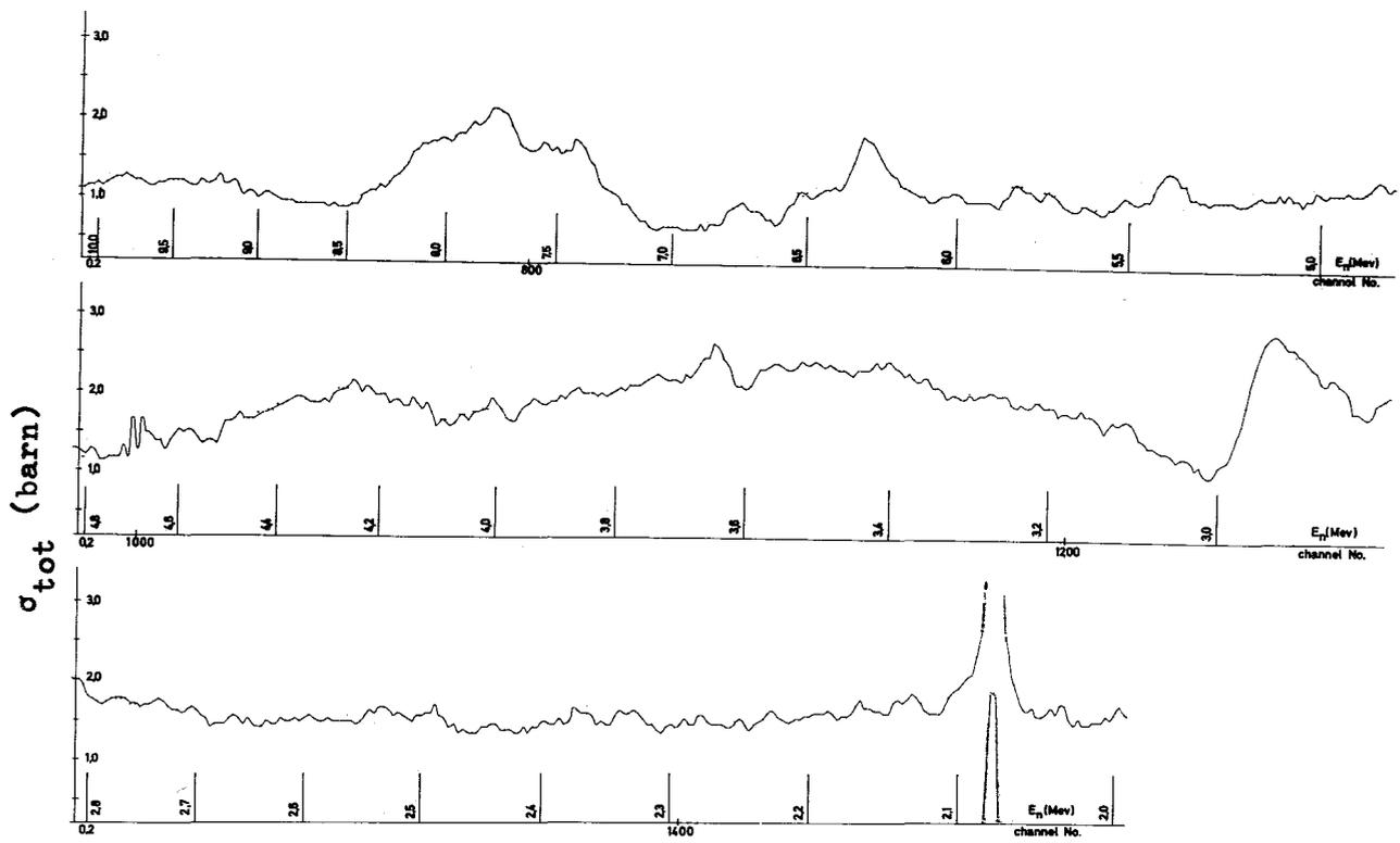
Fig. 4 - The total neutron cross-section of Carbon
