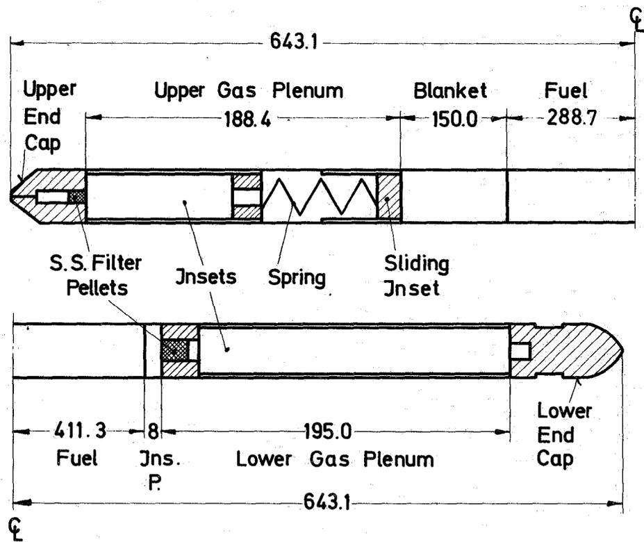
Fig. 3 The Pin Design (schematic)
