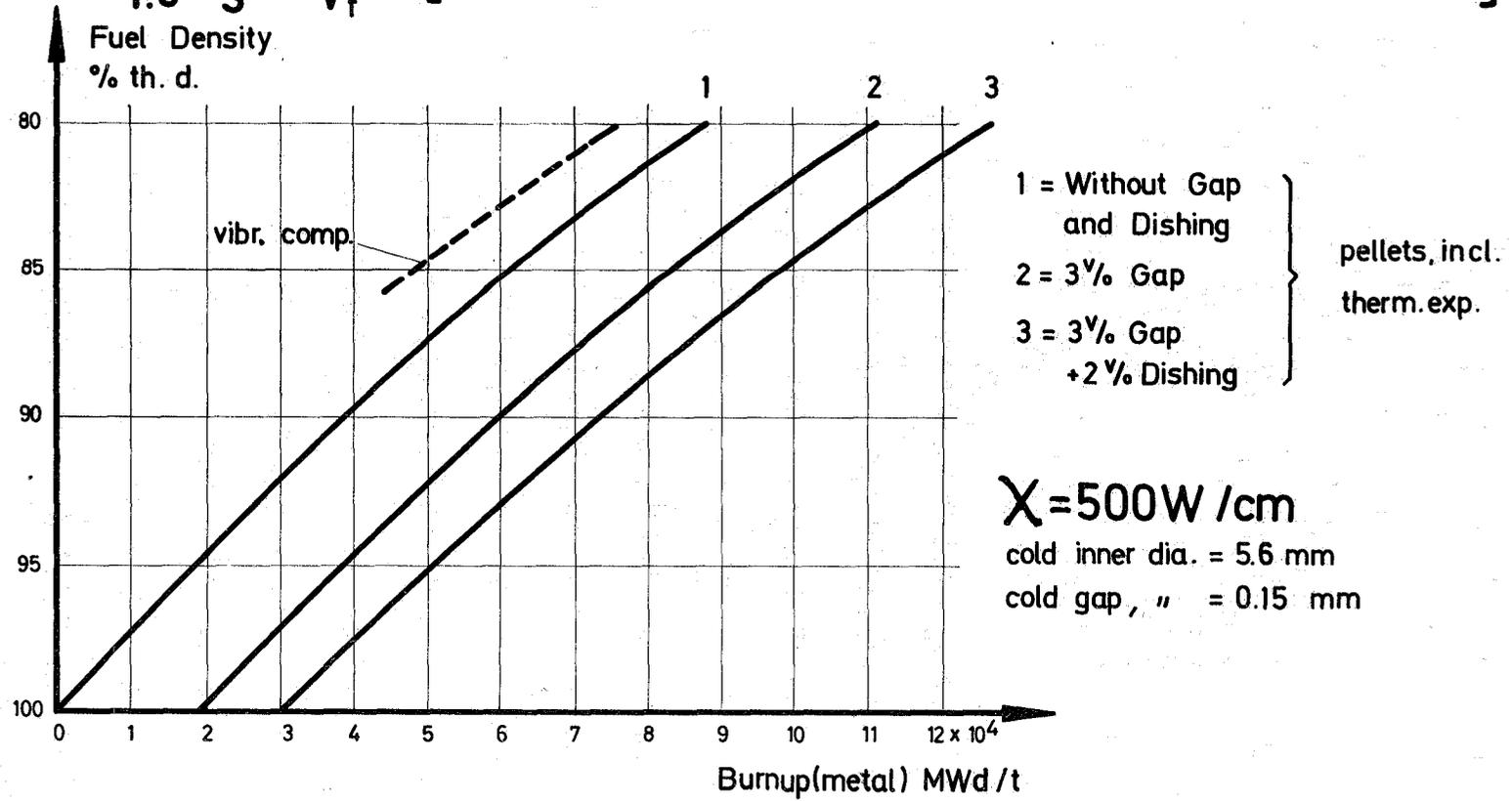
Fig. 1 Maximum Fuel Burnup Dependence on Density (cold)
