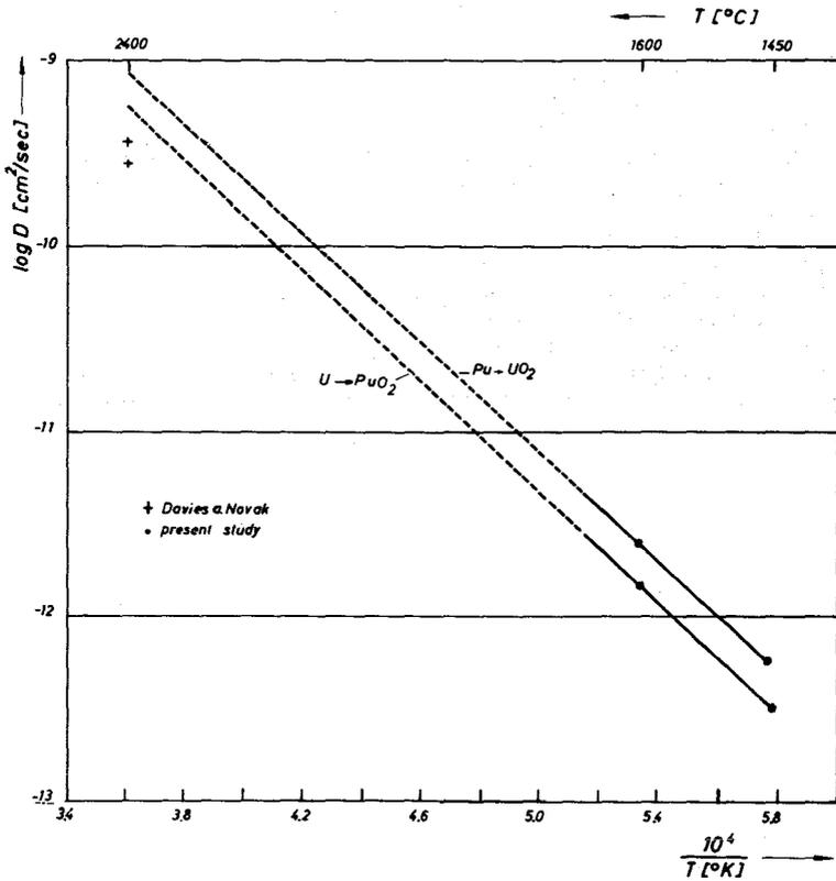
FIG. 6. Interdiffusion in mixed U, Pu oxides during sintering in Ar = 5% H<sub>2</sub>
