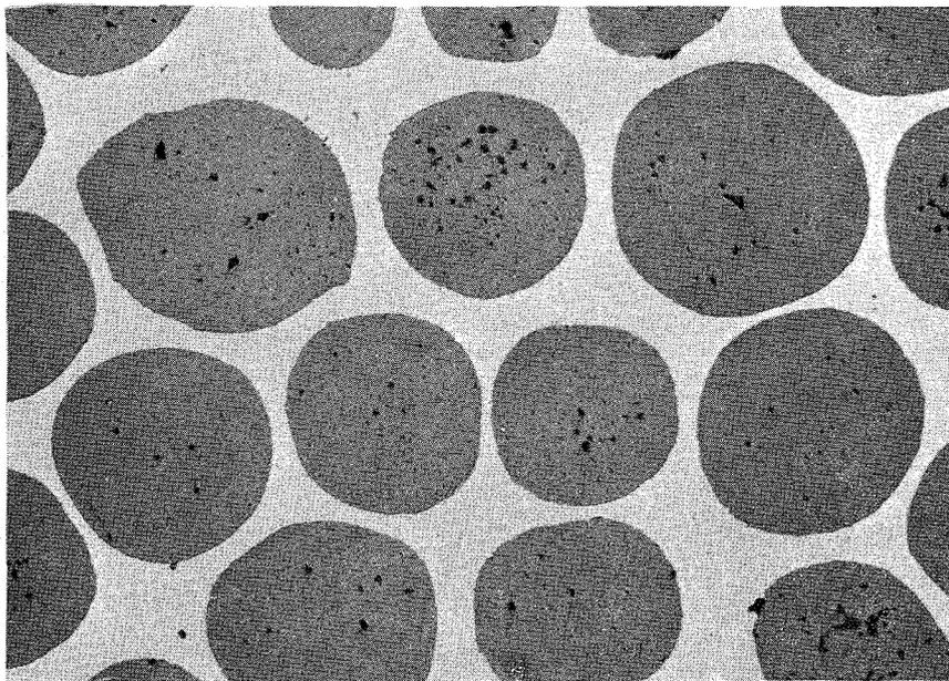
Fig. 3 Cylindrical specimen, hot compressed
