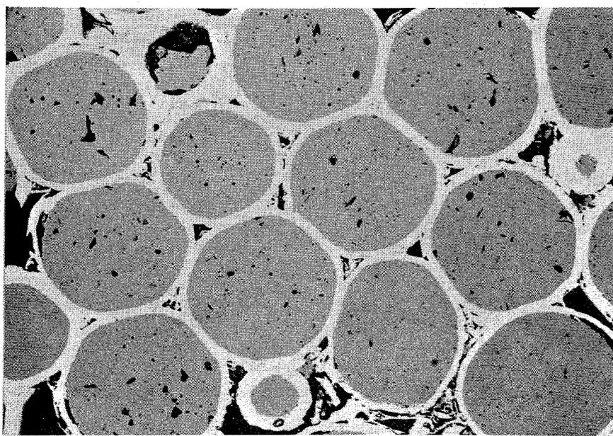
Fig. 2  $\text{UO}_2$  / 35 vol % Mo-cermet isostatically hot compressed
