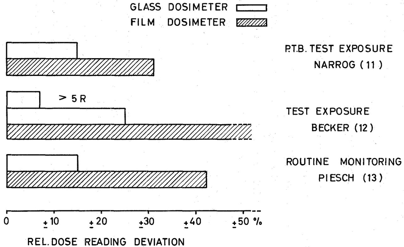
FIG.7. RESULTS OF INTERCOMPARISON MEASUREMENTS
