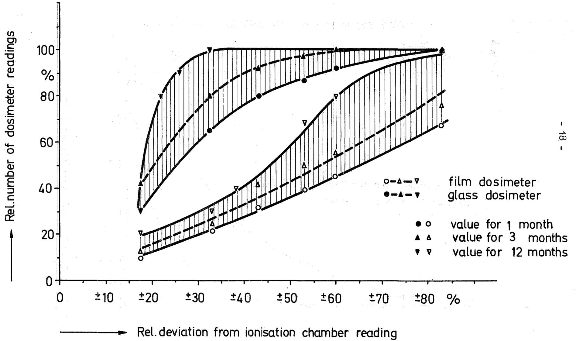
Tab. 6: Agreement of the measuring values related to the pocket chamber dosimeter
