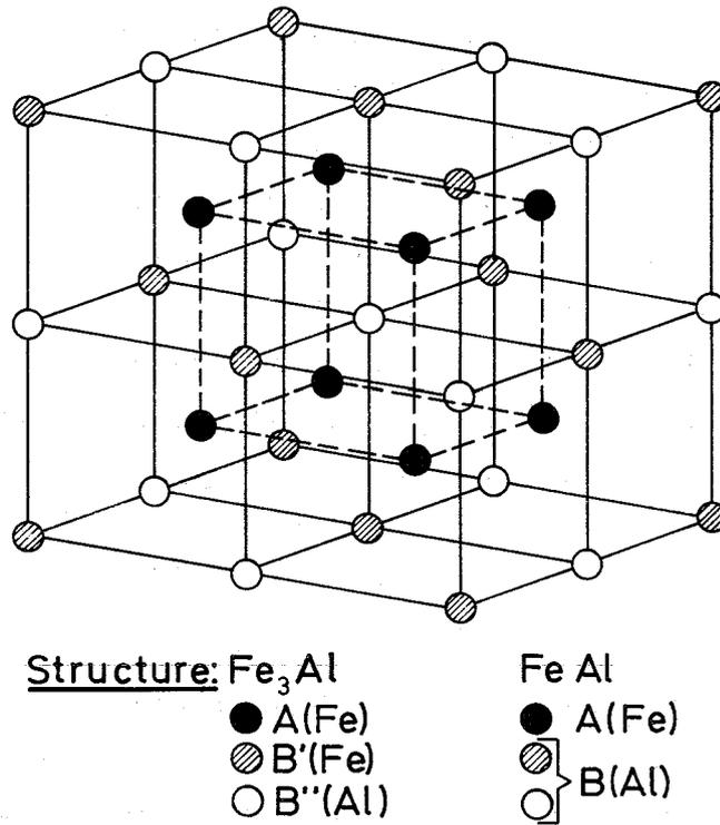
Fig. 1 Lattice structure and order of Fe - Al alloys
