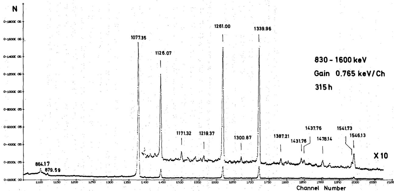
FIG. 1. Portion of the anti-Compton spectrum of  $^{67}\text{Zn}(n, \gamma)^{68}\text{Zn}$ .
