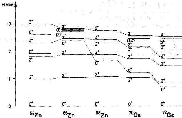
FIG. 5. Comparison between level schemes of even nuclei around  $A=68$  including all experimental data available in the literature.
