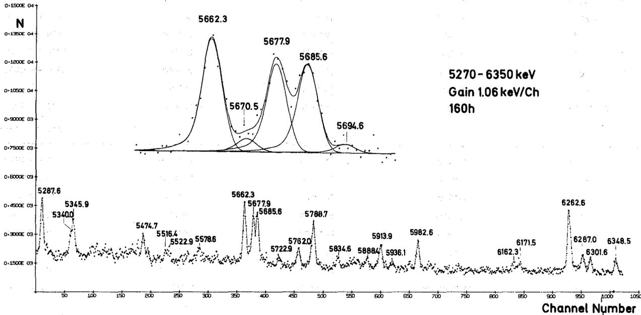
FIG. 2. Portion of the pair spectrum of  $^{67}\text{Zn}(n, \gamma)^{68}\text{Zn}$ .
