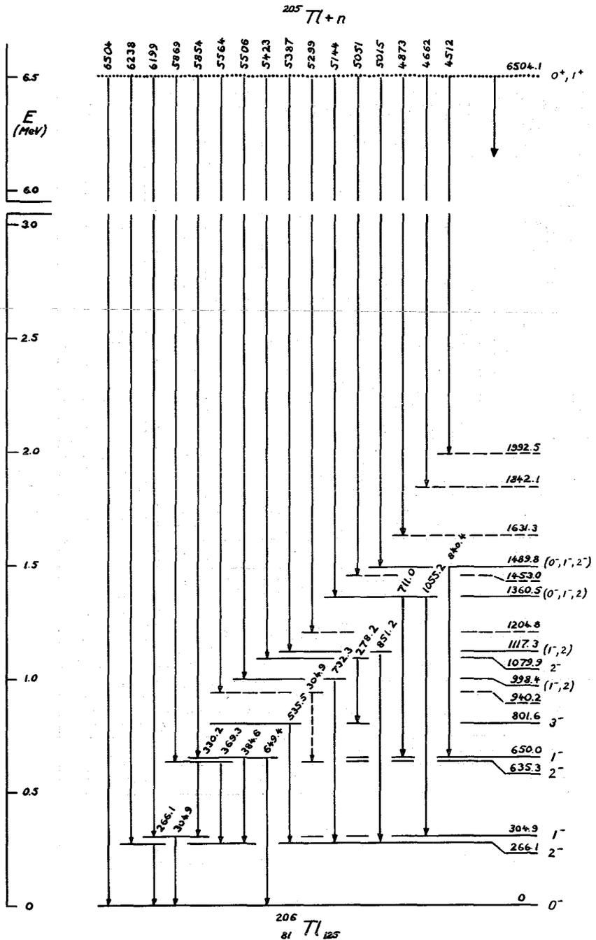
FIG. 4. Transition diagram of  $^{206}\text{Tl}$ .
