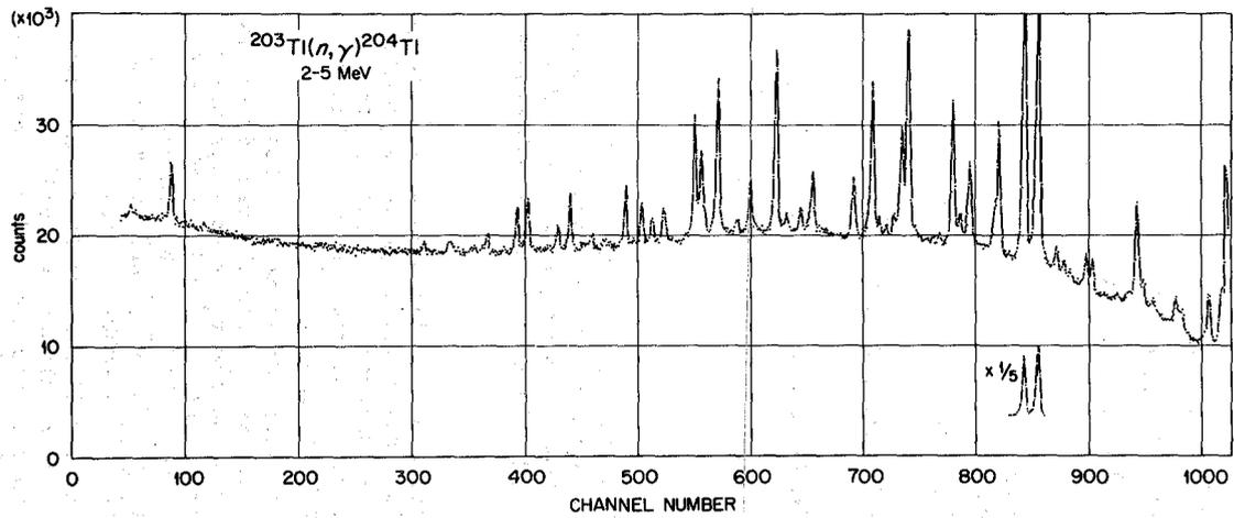
FIG. 2. High-energy part of the gamma spectrum from neutron capture in  $^{205}\text{Tl}$ .
