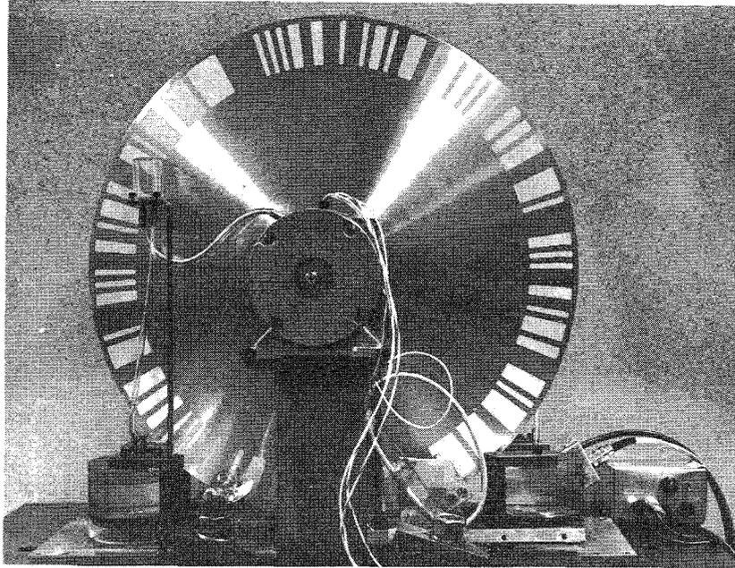
Fig.5 Statistical Chopping Wheel of Gompf et. al. [8]
