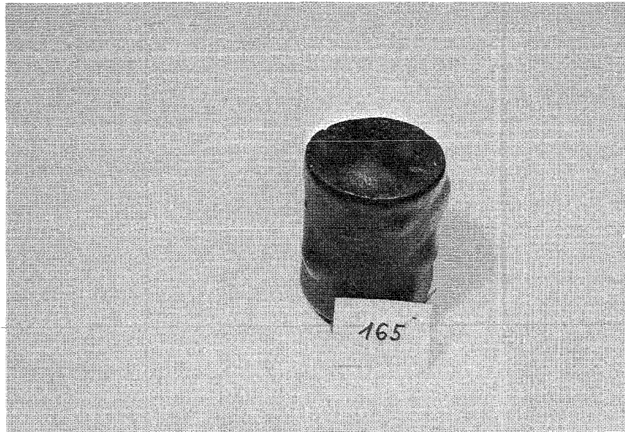
Fig. 2.3.3-1 Swelling of bitumen specimen 165 (19.25 % sodium carbonate, 19.25 % sodium nitrate in Mexphalt 15) after storage in distilled water (132 d). The water was changed corresponding to the leaching tests
