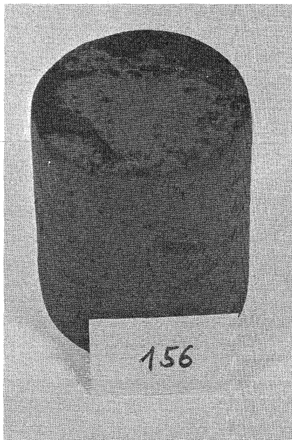
Fig. 2.3.3-5 Bitumen specimen 156 (19.25 % \text{NaNO}_3 , 19.25 % \text{NaOH} ) after storage in water for 309 days (no swelling).
