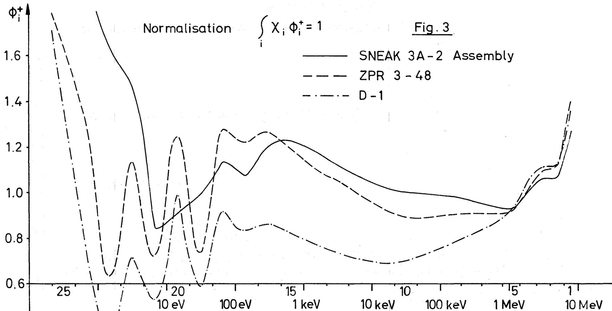
Comparison of adjoint flux spectra of SNEAK 3A-2 Assembly and D-1 Design.
