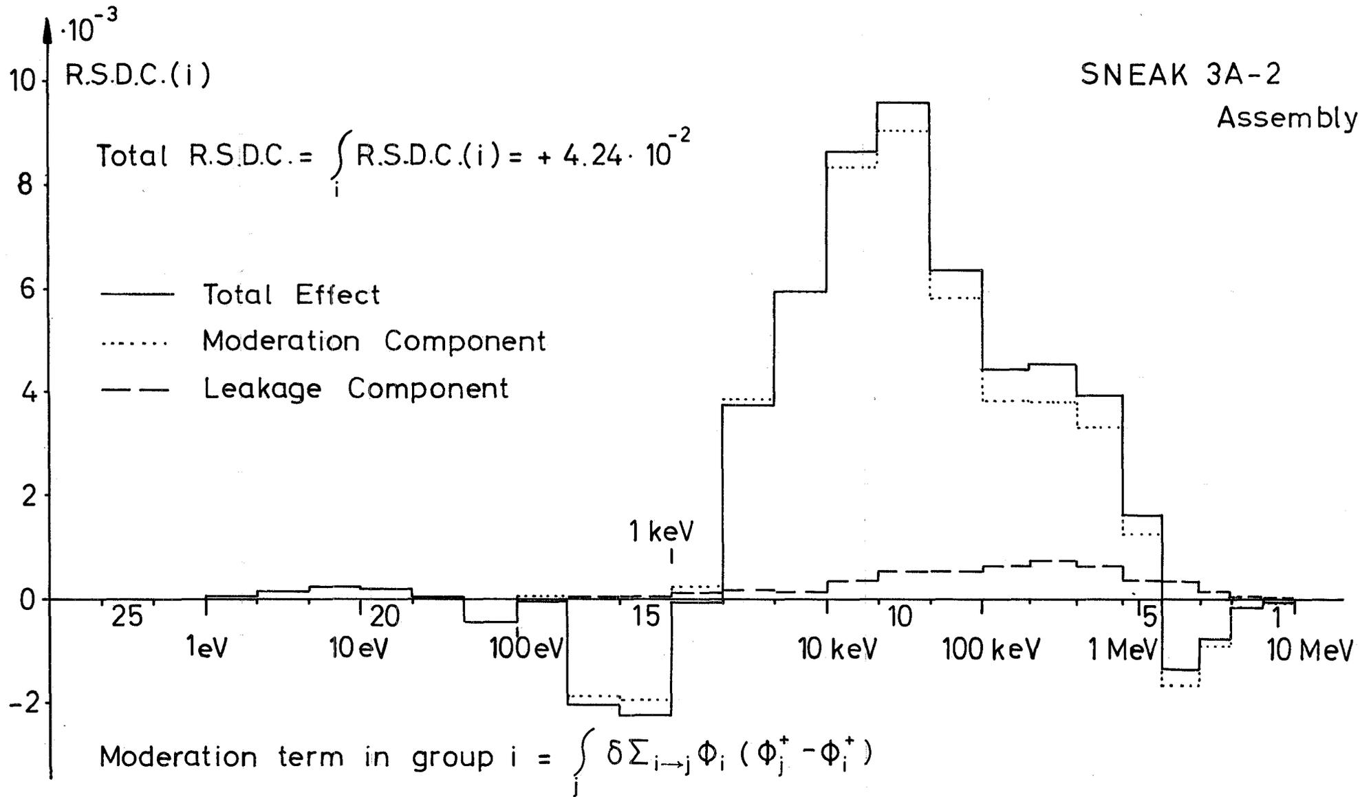
Energy dependence of the steam density coefficient for SNEAK 3A-2 Assembly
