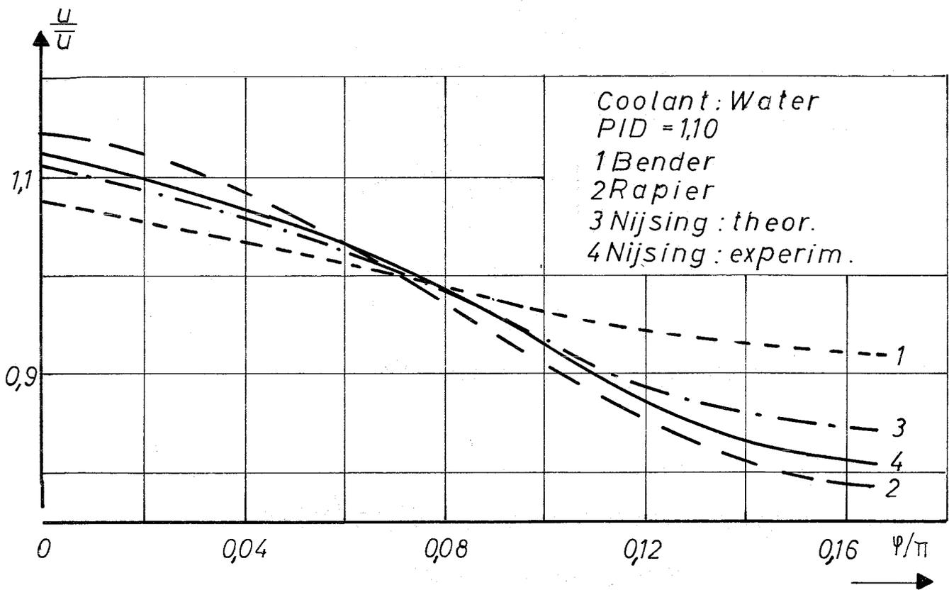
Fig2: Comparison of different relations for the eddy diffusivity  $\epsilon_{\phi M}$ .
