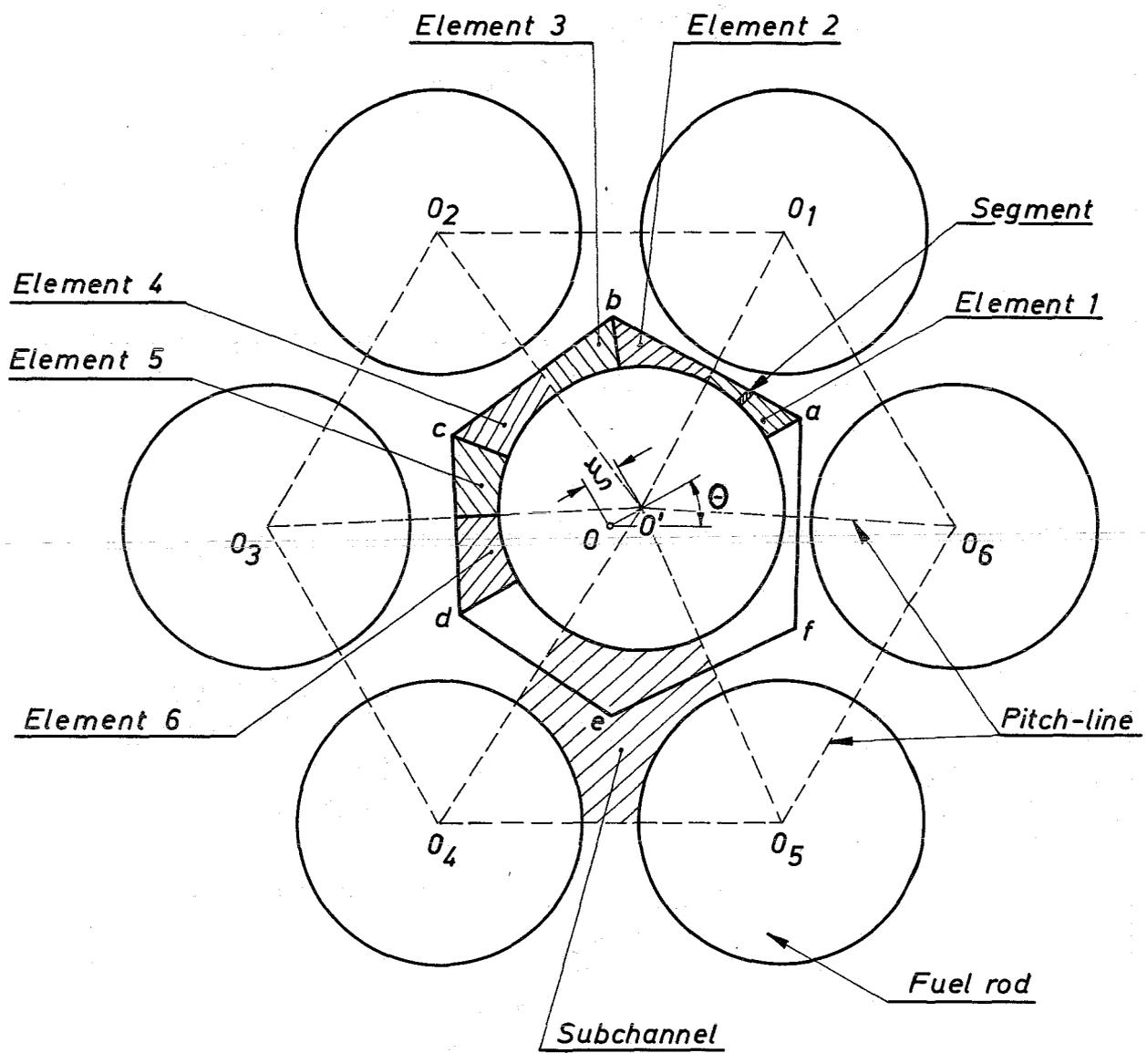
Fig 1: Cross-section of asymmetrical triangular rod cluster.
