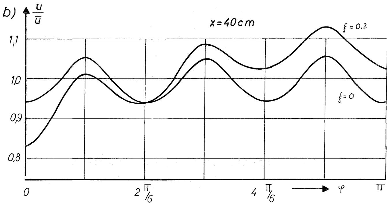
Fig 4: Flow velocity  $\frac{u}{U}$  vs angle  $\varphi$
