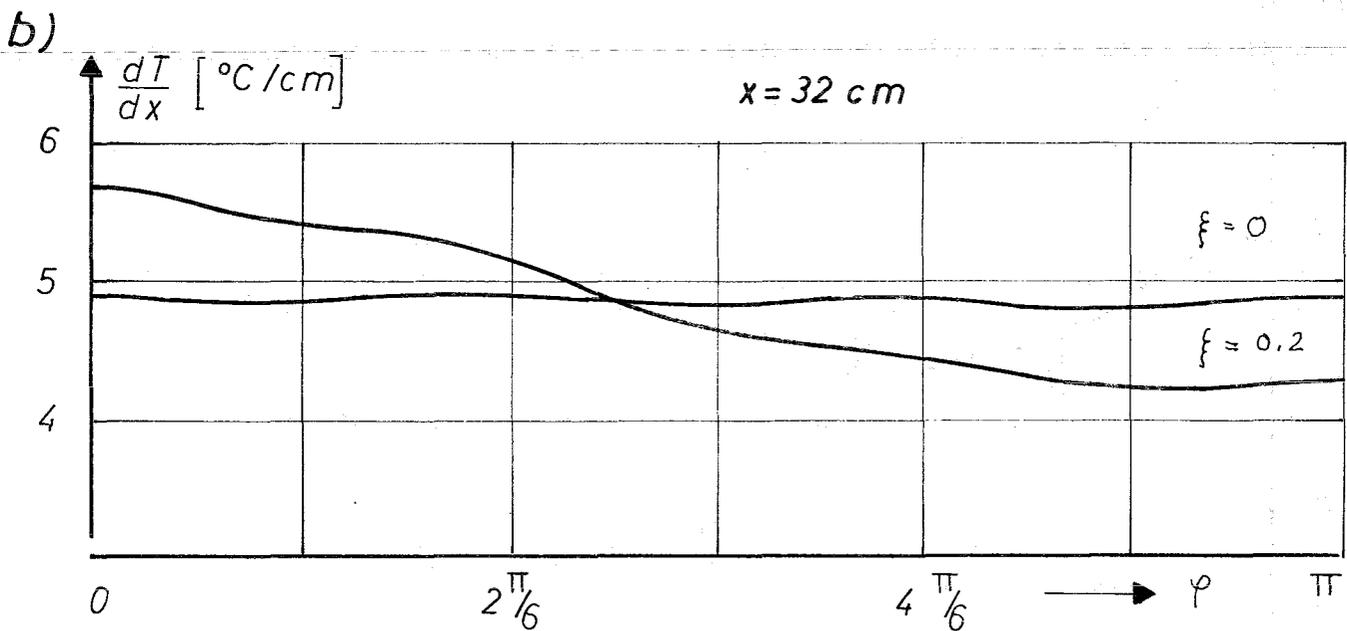
Fig 7: Axial temperature gradient  $\frac{dT_c}{dx}$  vs angle  $\varphi$
