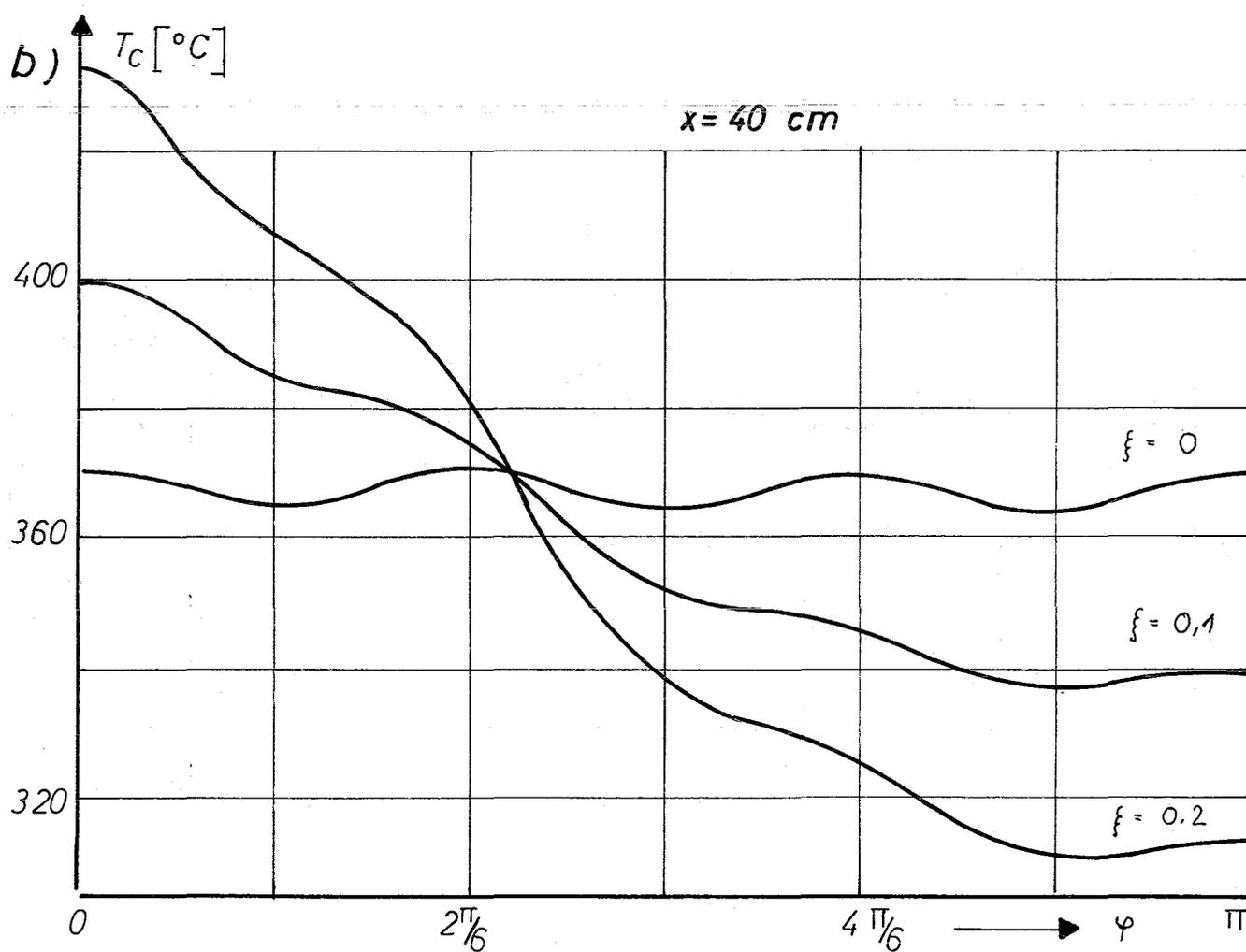
Fig 6: Coolant temperature  $T_c$  vs angle  $\varphi$
