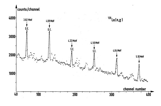
Fig. 8: Neutron capture  $\gamma$ -spectrum of <sup>139</sup>La, measured with a Ge(Li)-detector, target La<sub>2</sub>0<sub>3</sub>.
