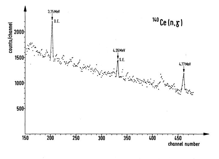
Fig. 4: Neutron capture γ-spectrum of <sup>140</sup>Ce, measured with a Ge(Li)-detector, target Ce<sub>2</sub>0<sub>3</sub>.
