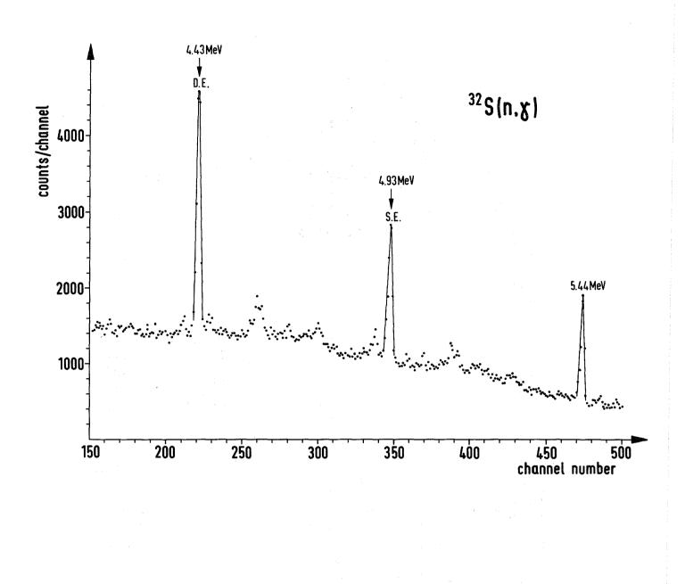
Fig. 2: Neutron capture  $\gamma$ -spectrum of  $^{32}$ S, measured with a Ge(Li) detector.
