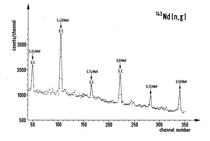
Fig. 6: Neutron capture  $\gamma$ -spectrum of <sup>143</sup>Nd, measured with a Ge(Li)-detector, target Nd<sub>2</sub>O<sub>3</sub>.
